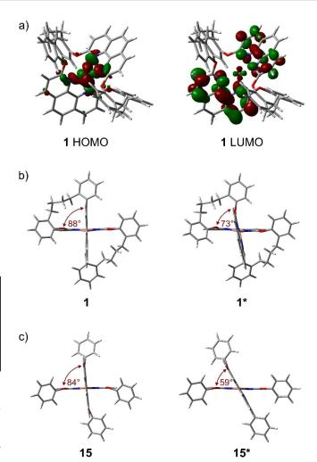
**Figure 4.** a) DFT-optimized structure of **1** at the B3LYP/LANL2DZ level of theory displaying the computed HOMO (left) and LUMO (right) orbitals. Comparison of computed ground-state (left) and excited-state geometries (right) of b) the macrocyclic complex **1** and c) the reference complex **15** (bottom). The angles measured between both phenanthroline planes are given in ruby red.
