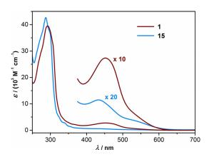
**Figure 3.** UV/Vis spectra of the macrocyclic complex **1** and the reference complex **15** measured in acetonitrile at room temperature. To improve their visibility, the MLCT absorption bands in the visible were increased by the indicated scaling factors.
