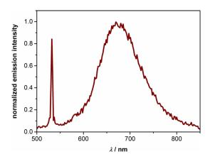
Figure 5. Emission spectrum of complex 1 in frozen CH<sub>3</sub>CN matrix at 77 K after excitation at 532 nm with laser pulses of  $\approx$  10 ns duration. The spectrum was time-integrated over 100 ns starting with the laser pulse (pulse energy, 30 mJ). The sharp peak at 532 nm is due to stray excitation light.
