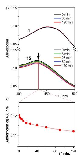
**Figure 6.** a) UV/Vis data of 1 (top) and 15 (bottom) recorded after different periods of LED illumination (455 nm, 500 mW optical output) to investigate photostability. b) Development of the absorption of 15 at 433 nm during the experiment.
