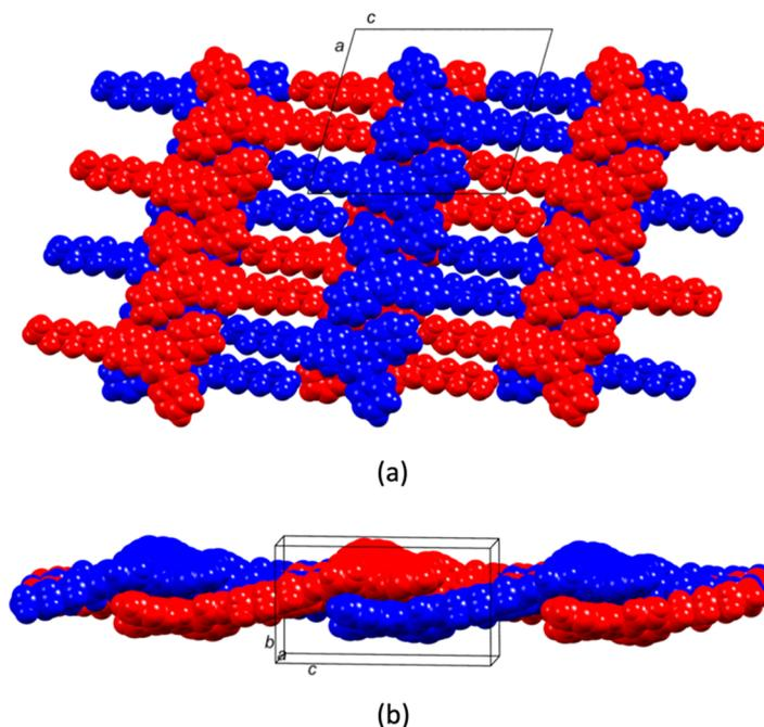
**Figure 5.** Part of two interwoven supramolecular sheets showing how the voids in one sheet (see Figure 4b) are occupied by *n*-hexyloxy chains from the next sheet. (a) Viewed down the *b*-axis, and (b) viewed approximately down the *a*-axis.
