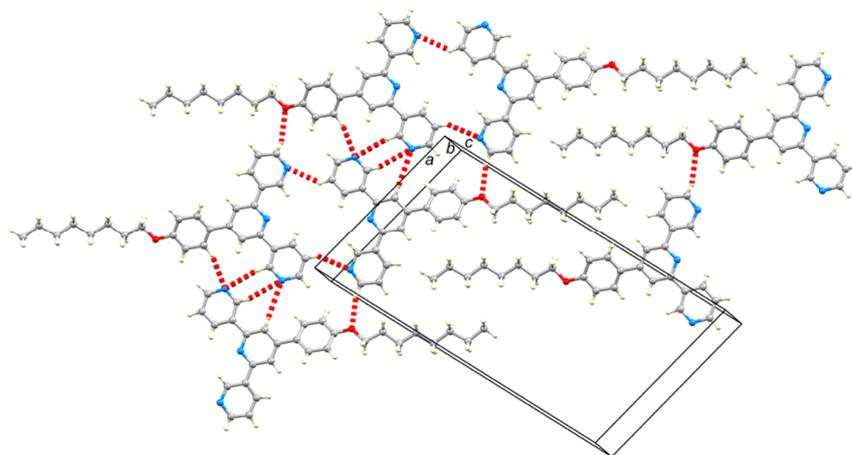
**Figure 8.** Within each layer of molecules of **8**, van der Waals interactions between *n*-alkyloxy chains, and C–H...N and C–H...O weak hydrogen bonds (red hashed lines) are important packing interactions. See Figure S15 for a space-filling representation.
