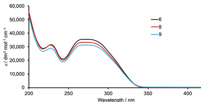
**Figure 1.** The solution absorption spectrum of compounds **6**, **8** and **9** (MeCN, see Table 2).
