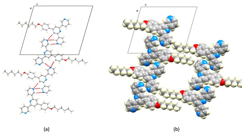
**Figure 4.** Molecules of **6** pack into 2D-sheets involving CH...N weak hydrogen bonds and van der Waals interactions between *n*-hexyloxy chains. The unit cell is viewed down the *b*-axis. (a) C–H...N hydrogen bonds and (b) a space-filling representation of part of one supramolecular sheet showing one void between pairs of *n*-hexyloxy chains.
