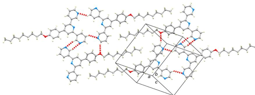
**Figure 10.** Packing of molecules of **9** within one 2D-sheet involves a combination of C–H...N and C–H...O weak hydrogen bonds (red hashed lines) and van der Waals interactions between *n*-nonyloxy chains. Figure S16 (in the Supplementary Materials) shows this packing in a space-filling representation.
