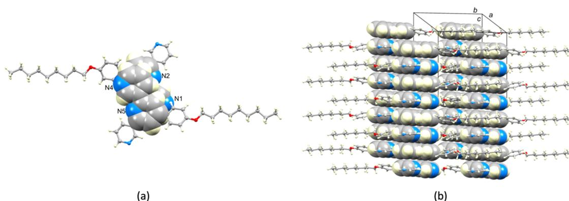
**Figure 9.** (a) Offset face-to-face  $\pi$ -stacking of two crystallographically independent molecules of **9**. (b) Packing of molecules of **9** into 2D-layers with the  $\pi$ -stacking shown in (a) highlighted in space-filling representation.
