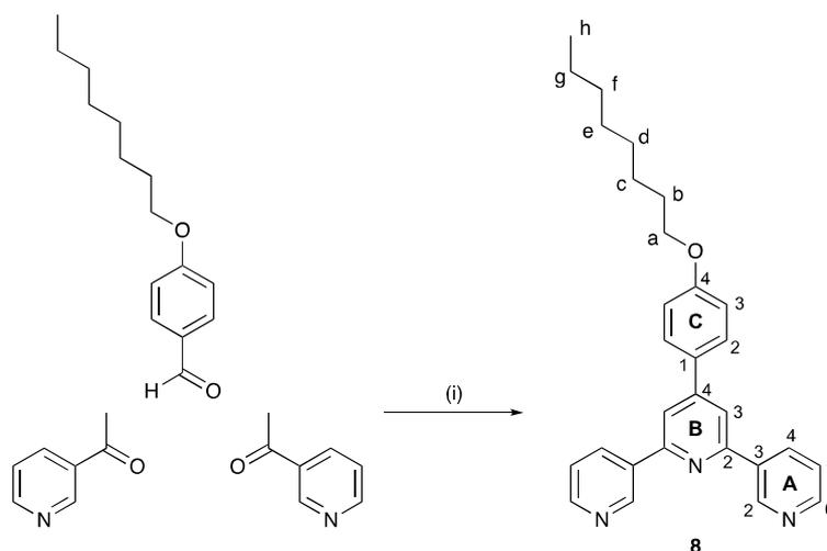
**Scheme 2.** Synthesis of compound **8**; **9** was prepared in a similar manner. Conditions: (i) KOH, EtOH;  $\text{NH}_3$  (aqueous), room temperature. The numbering scheme for NMR assignments is shown; an analogous scheme is used for **9**.
