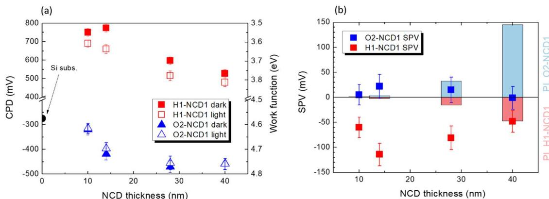
**Figure 3.** Contact potential difference (CPD) dependence on NCD1 thickness, surface chemistry, and illumination (a). Surface photovoltage (SPV) dependence on NCD thickness and surface chemistry. SiV PL intensity is shown as red (H1-NCD1) and blue (O2-NCD2) bars (b).
