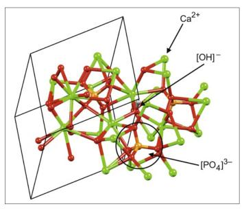
Fig. 3. The unit cell of hydroxyapatite with part of the 3-dimensional structure. Ca<sup>2+</sup> ions are shown in green, the OH unit is directed along the crystallographic *c*-axis, and one  $[PO_4]^{3-}$  ion is highlighted (P, orange; O, red). [Data: R.T. Downs, M. Hall-Wallace, The American Mineralogist Crystal Structure Database, *Amer. Mineral.* **2003**, *88*, 247.]
