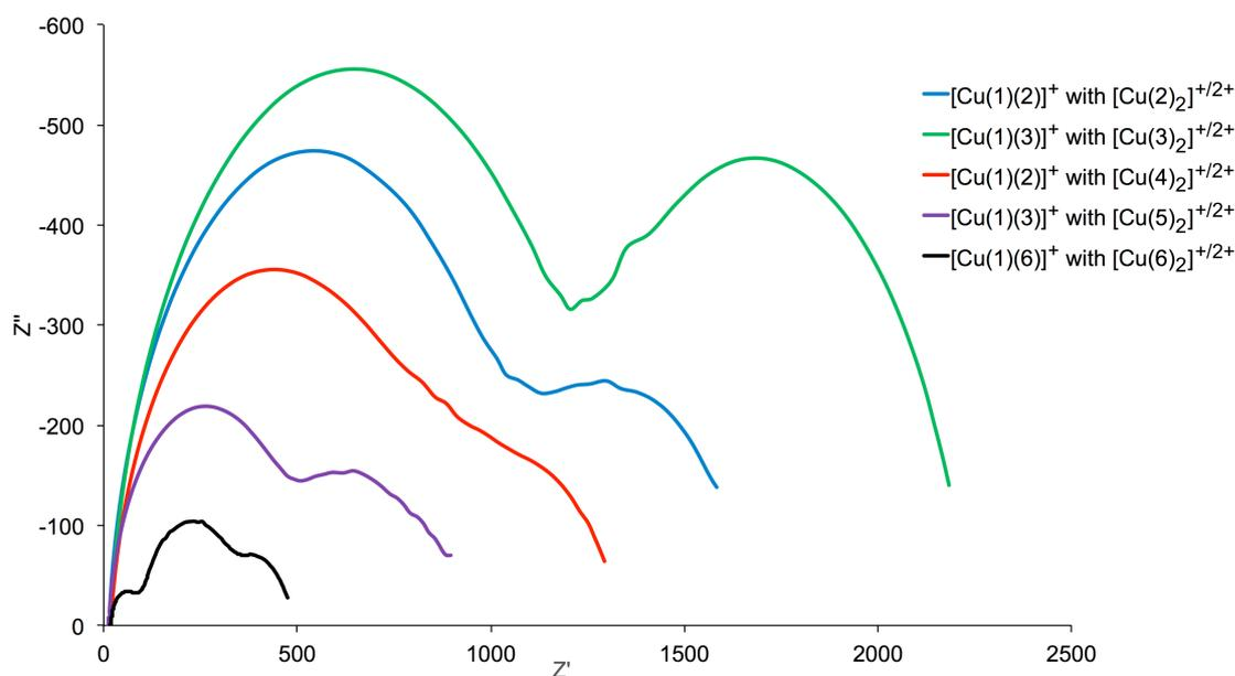
**Fig. 5.** Nyquist plots for DSCs containing the best-performing combination of dye and each electrolyte.
