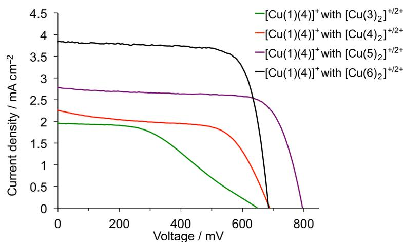
**Fig. 2.**  $J$ - $V$  curves for the DSCs containing the dye  $[\text{Cu}(1)(4)]^+$  and electrolytes  $[\text{Cu}(3)_2]^{+/2+}$ ,  $[\text{Cu}(4)_2]^{+/2+}$ ,  $[\text{Cu}(5)_2]^{+/2+}$ ,  $[\text{Cu}(6)_2]^{+/2+}$  on the day of sealing the DSCs.
