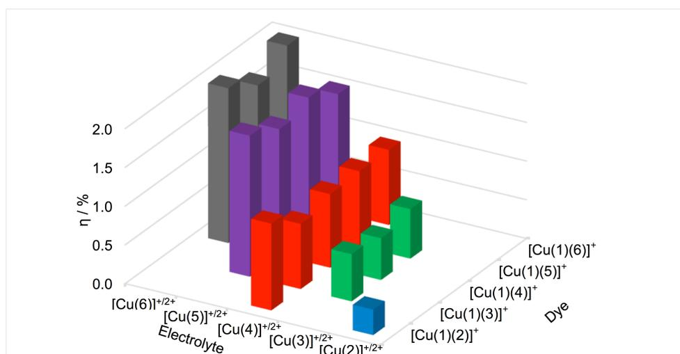
**Fig. 4.** Photoconversion efficiencies of the DSCs in Table 3 as a function of ancillary ligand and electrolyte.
