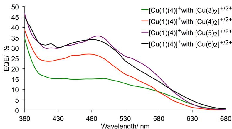
**Fig. 3.** EQE spectra for the DSCs containing the dye  $[\text{Cu}(1)(4)]^+$  and electrolytes  $[\text{Cu}(3)_2]^{+/2+}$ ,  $[\text{Cu}(4)_2]^{+/2+}$ ,  $[\text{Cu}(5)_2]^{+/2+}$  or  $[\text{Cu}(6)_2]^{+/2+}$  recorded 1 day after sealing the DSCs.
