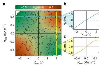
**Figure 3 | Influence of a V<sub>2</sub>O<sub>3</sub> buffer layer on Cr<sub>2</sub>O<sub>3</sub> magnetoelectricity.** (**a**) Magnetoelectric field cooling map of the antiferromagnetic order selection for a V<sub>2</sub>O<sub>3</sub>/Cr<sub>2</sub>O<sub>3</sub>/Pt system. (**b**,**c**) Line profiles taken from the map in **a**. Only non-zero products of gate voltage and magnetic field lead to appreciable order parameter selection, whereas the individual stimuli do not.
