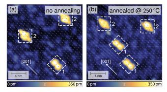
FIG. 3. Constant current STM images of ZnTPP on rutile TiO<sub>2</sub> (110): (a) after evaporation to the cold substrate ( $V_{sample} = 1.8 \text{ V}$ ,  $I_t = 20 \text{ pA}$ ) and (b) after 30 min annealing to 250 °C ( $V_{sample} = 1.8 \text{ V}$ ,  $I_t = 10 \text{ pA}$ ).
