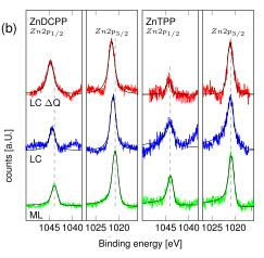
FIG. 5. PES spectra of ZnDCPP and ZnTPP on rutile  $TiO_2$  (110) for submonolayer coverage after deposition (LC), after annealing (LC $\Delta$ Q), and multilayer (ML) coverage: (a) Valence band spectra obtained with a photon energy of hv = 65 eV. (b) PES of Zn2p obtained with a photon energy of hv = 1253 eV. The dashed lines indicate the position of the highest occupied molecular orbitals. The graphs at the bottom show the changes upon annealing.
