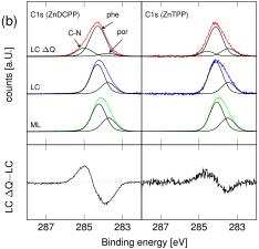
FIG. 6. PES spectra of ZnDCPP and ZnTPP on rutile  $TiO_2$  (110) for submonolayer coverage after deposition (LC), after annealing (LC $\Delta$ Q), and multilayer (ML) coverage: (a) N 1s spectra obtained with a photon energy of  $h\nu = 500$  eV. (b) C 1s spectra obtained with a photon energy of  $h\nu = 340$  eV. The bottom graph shows the relative difference between the just deposited molecules and after annealing.
