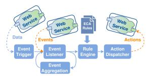
Figure 2: Condition Action System connects to Web services. Web services deliver data to the Event Trigger or events to the Event Listener. Subsequently, the Rule Engine processes events according to predefined ECA Rules and instructs the Action Dispatcher for further actions.
