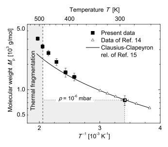
FIG. 4. The crucible temperature dependence of the peak molecular weight  $M_p$  of vinyl-terminated PDMS polymer (filled squares) is compared with derived vapor pressure data of trimethyl-terminated PDMS from Lei *et al.* (Ref. 16) (open triangles) and from Wilcock (Ref. 17) (line). Gray shading marks the boundaries of thermal fragmentation (dashed line) and the background gas pressure (dotted line).
