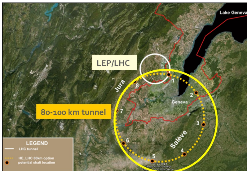
Figure 2. A possible implementation of the 80 km tunnel (dashed circle) that would host TLEP and the VHE-LHC in the Geneva area, taken from ref. [10]. The 100 km version (full line) is currently under study.
