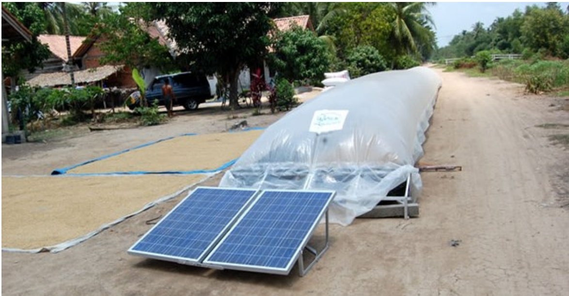
Figure 9.3 Solar Bubble Dryer (center) next to traditional drying of rice on the side of the street (left) Source: IRRI Rice Knowledge Bank (2021e)
