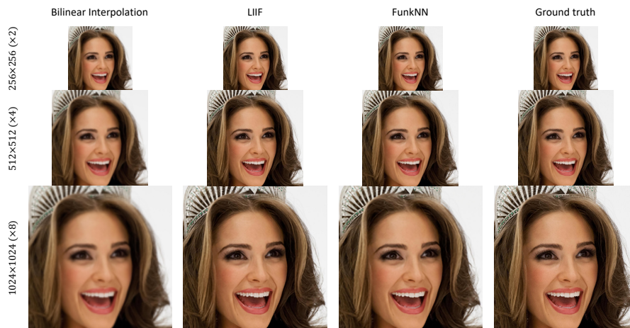
Figure 4.4: FunkNN model is only trained over CelebA-HQ images of maximum resolution 128 \times 128 , but it can reliably reconstruct high-quality images in higher resolutions.
