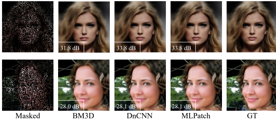
Figure 2.8: Comparison on image in-painting ( p = 30\% ) in resolution 128 \times 128 for PnP algorithm with different denoising priors.
