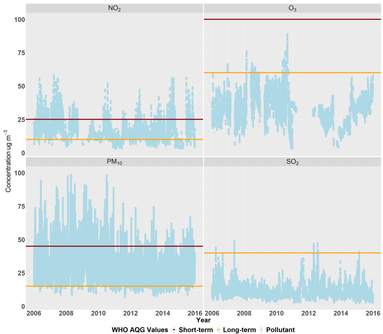
Figure S 2: Daily mean concentrations of PM 10 , NO 2 , SO 2 and O 3 in Cape Town, 2006 – 2015. The horizontal lines show the WHO AQG 2021 values for short-term (black) and long-term (orange) of each pollutant.
