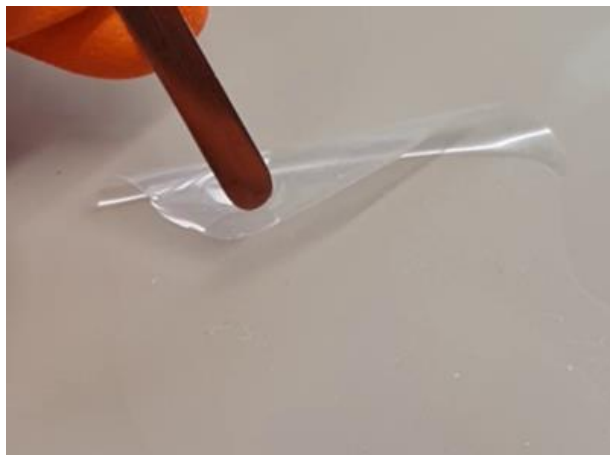
Figure 9-13. Picture of the self-standing thin film obtained from the self-assembled micelle solution (difficult to handle).
