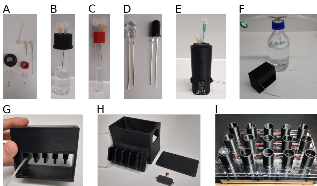
Figure 3.10: Components of the Aionostat. A: Needles, silicon tubing, Luer connector, open vial caps, silicon septum and magnetic stir bars used in the assembly of the vials. B: Big vial assembly (40mL). C: Small vial assembly (8mL). D: LED and phototransistor for the bacterial density measurement. E: Full assembly of one vial in its vial holder. F: Pump connection to the input bottle. G-H: piezoelectric pump array and housing (5 pumps version). I: Vial holders positioned on the magnetic stirring plate.
