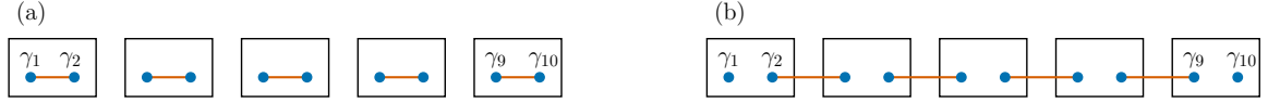
Figure 1.1: Kitaev chain with five fermionic sites : (a) If the hopping amplitude and the superconducting pairing potential are set to zero, then only Majorana modes (blue dots) from the same fermionic site (black rectangle) are paired. (b) In contrast, if the system is tuned to the limit of vanishing chemical potential and a pairing potential that is equal to the hopping amplitude, then only Majorana operators from different sites couple. This means for a chain with open boundary conditions that the Majorana mode at the very left ( \gamma_1 ) and the very right ( \gamma_{10} ) remain unpaired and together form a nonlocal fermionic state.
