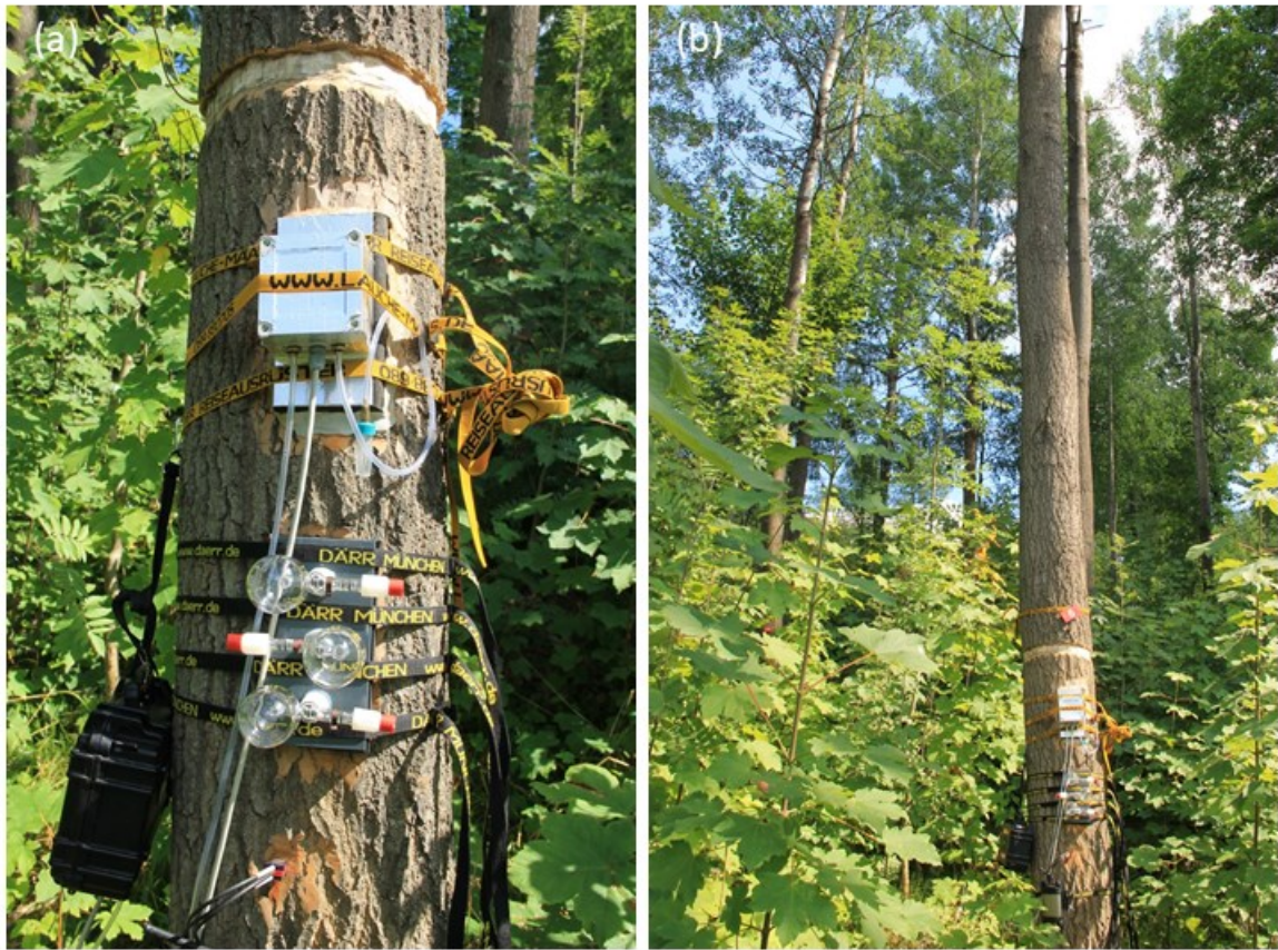
Picture S2 Experimental set-up with the respiration chamber below the girdling, the glass flasks for gas sample analysis and Sap Flow Meter SFM1 in 2018.
