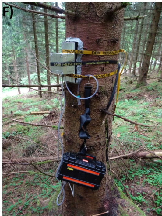
S3 A) and B) Calibration and testing unit for 10 COZIR and 10 LuminOx sensors. C) Sensor box for COZIR and LuminOx sensors covered with aluminium foil, D) COZIR and LuminOx sensors placed inside the waterproof housing. E) Sensor box and base plate of the chamber module and F) Installation in the field with sensor box and waterproof transport-case.
