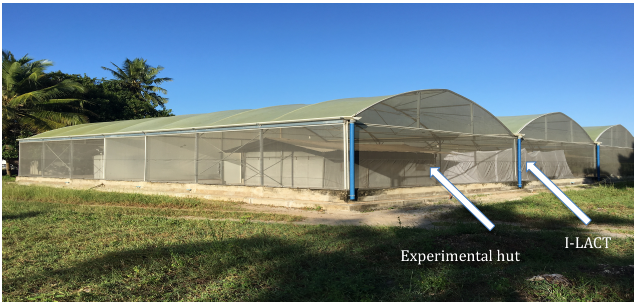
Figure 5.1. image of the Semi-field System with Large Ifakara ambient Chamber Test (I-LACT) measured (6x6x2 m). in each compartment
