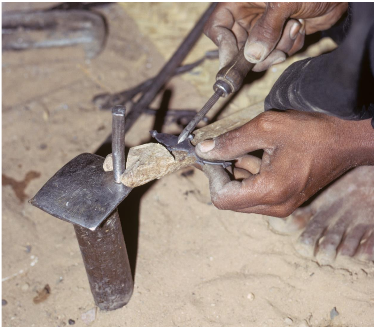
Fig. 55: After filing, the piece of jewellery is slightly annealed in the fire to darken the silver surface. This makes it easier to observe the chasing work that now follows with the graver (cf. fig. 19). The graver has a sharp, lancet-shaped end with which very fine zigzag lines can be engraved into the silver (fig. 20). To do this, the graver must be pushed back and forth with a measured amount of force: A "tremolo" stitch is created.
