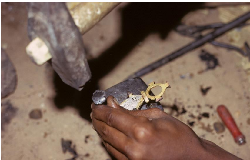
Fig. 49: The silver casting is exposed and shows the rough, yellowish "casting-skin". This must now be filed and polished. First, the sprue funnel (casting pin; Figs. 25 and 28) is cut off with the chisel (photo).
