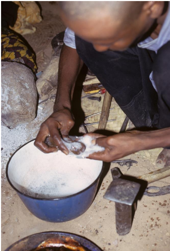
Fig. 60: After "white boiling", the silver object is "scraped" in a soapy water with a brush and brought to a high gloss. Hamid: "L'Omo [detergent] de Nigéria polit mieux que l'Omo du Niger".
