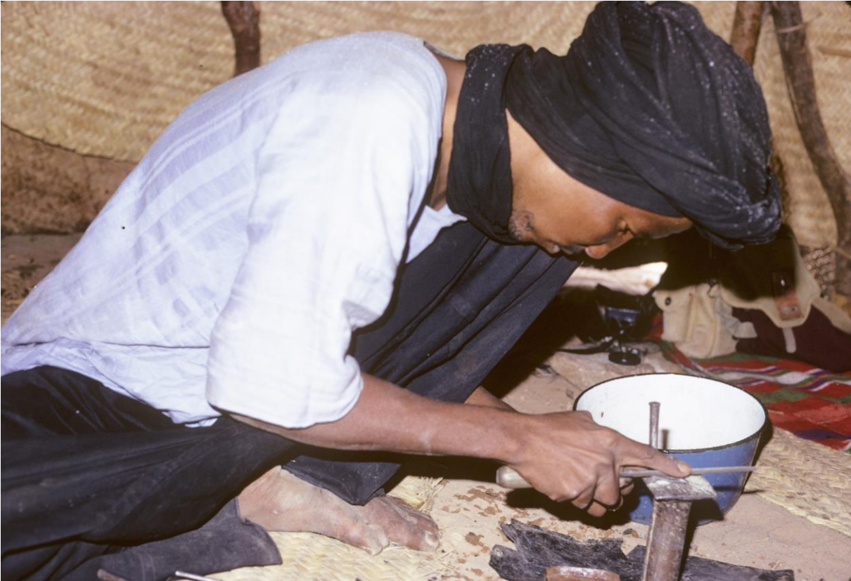
Fig. 52: With the cast blank, the work on an Agadez or Iférouane cross is only half finished! Now the piece has to be elaborately "trimmed", first by fine filing of all surfaces (photo), then by fine grinding, "white boiling" and polishing. Fine sanding is done with sandpaper, which has to be bought on the market.
