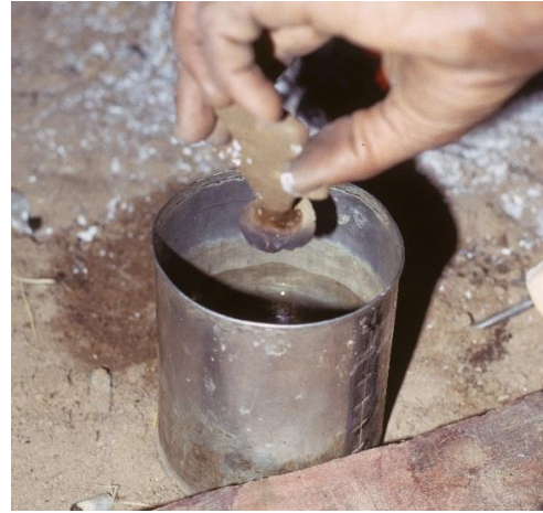
Fig. 33: As soon as the valuable beeswax in the mould is liquid, it is poured out in water and reused later.
