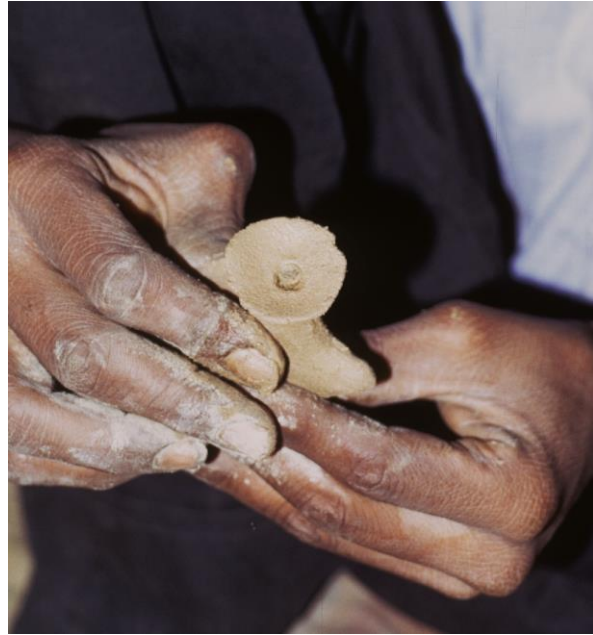
Fig. 27: The sprue funnel is modelled at the lower end of the Iférouane cross, in extension of the sprue funnel.
