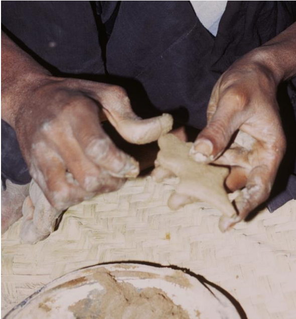
Fig. 26: The clay mould is finished and carefully smoothed. It is still wet.
