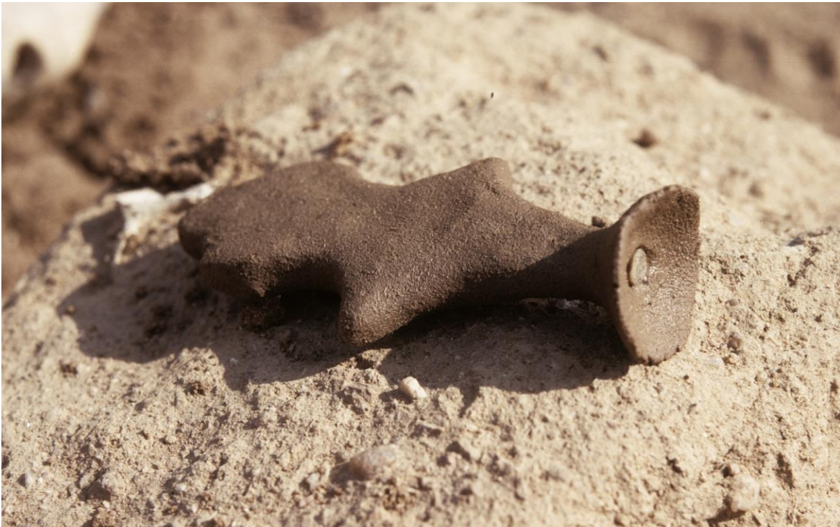
Fig. 28: The clay mould is finished and completely fitted with the sprue funnel (right). It is placed in the sun to dry for a few hours. The thin wax funnel is visible in the centre of the clay funnel.
