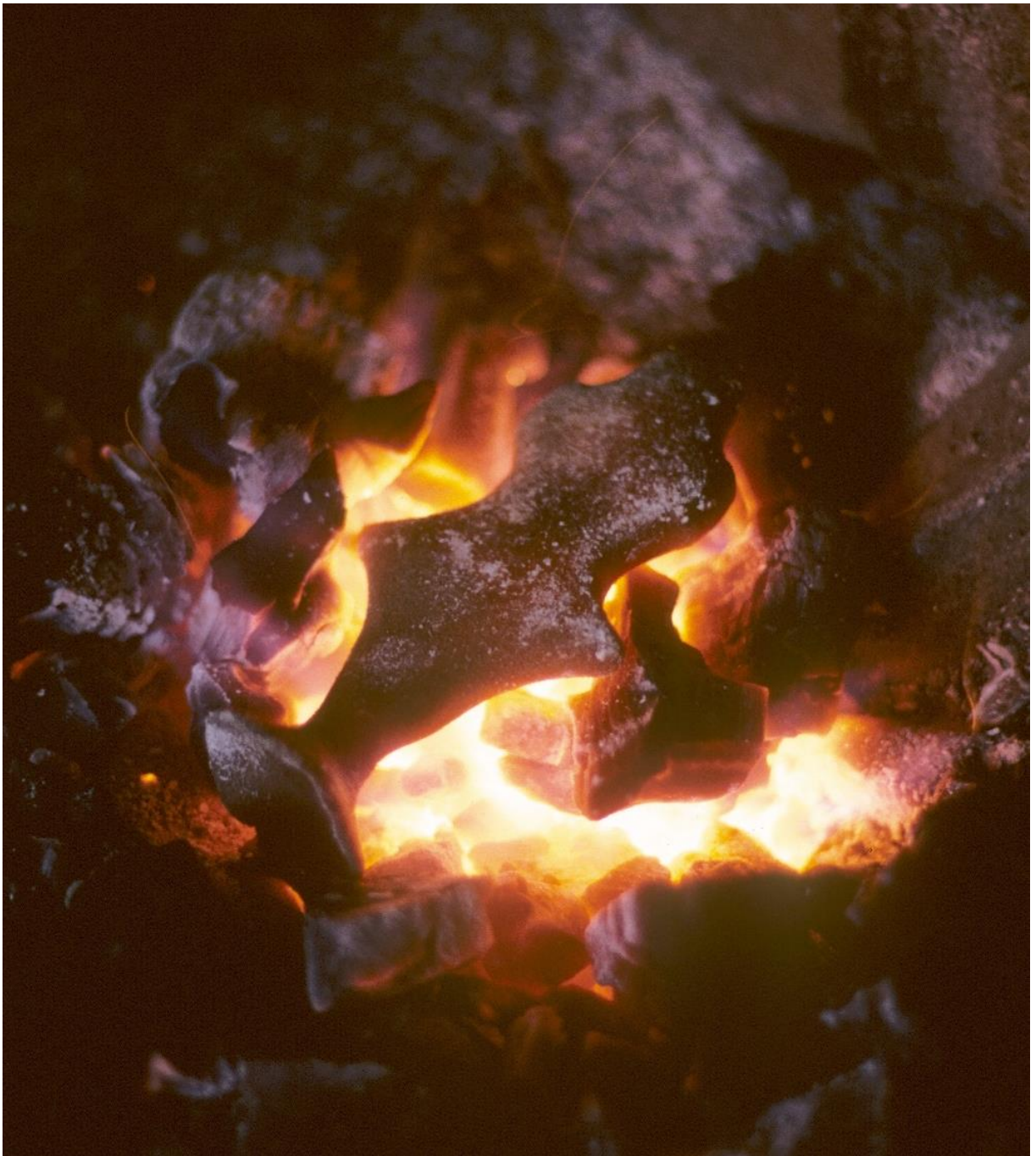
Fig. 40: The mould is fired – still without the attached, filled crucible.
