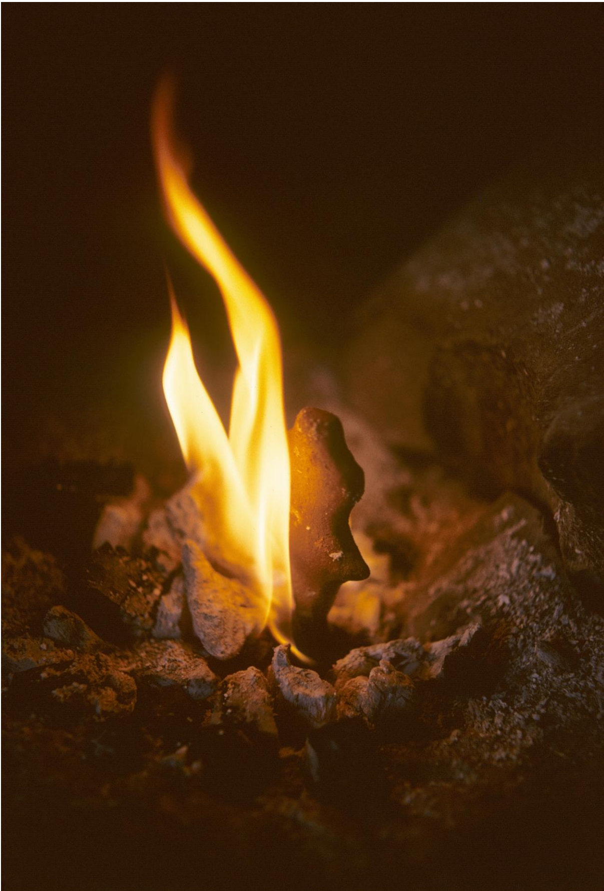
Fig. 43: Now the mould is fired "upside-down" in a hot charcoal fire – like ceramics. Only in this way will it survive the heat shock of pouring in the liquid silver at around 900–1000° C without bursting. The crucible is hidden at the bottom in the glowing charcoals; the mould attached to the top protrudes but is also heated thoroughly.
