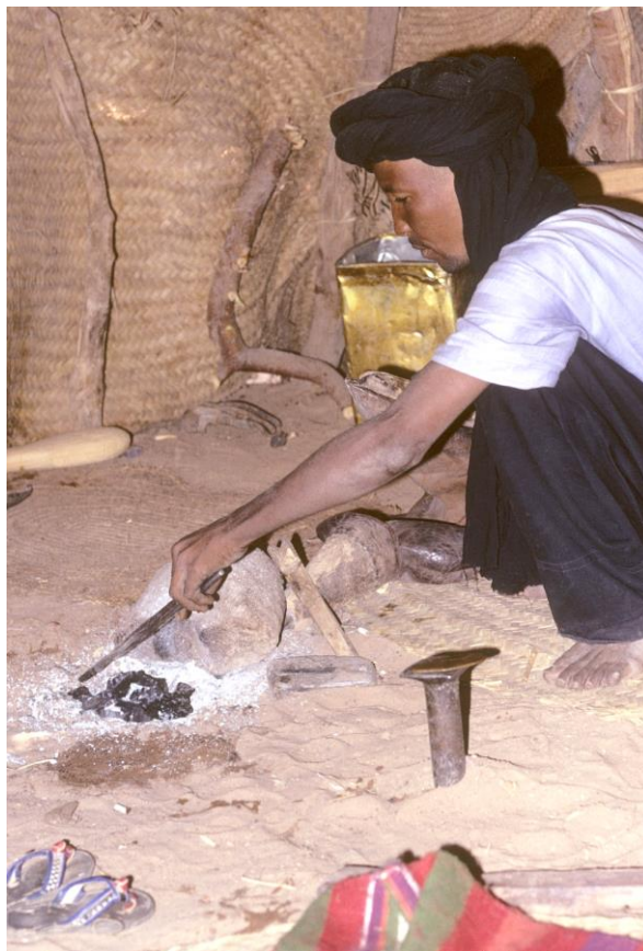
Fig. 29: In the meantime, Hamid stokes the charcoal fire again and prepares it to melt out the wax and then to pre-fire the empty cast mould.
