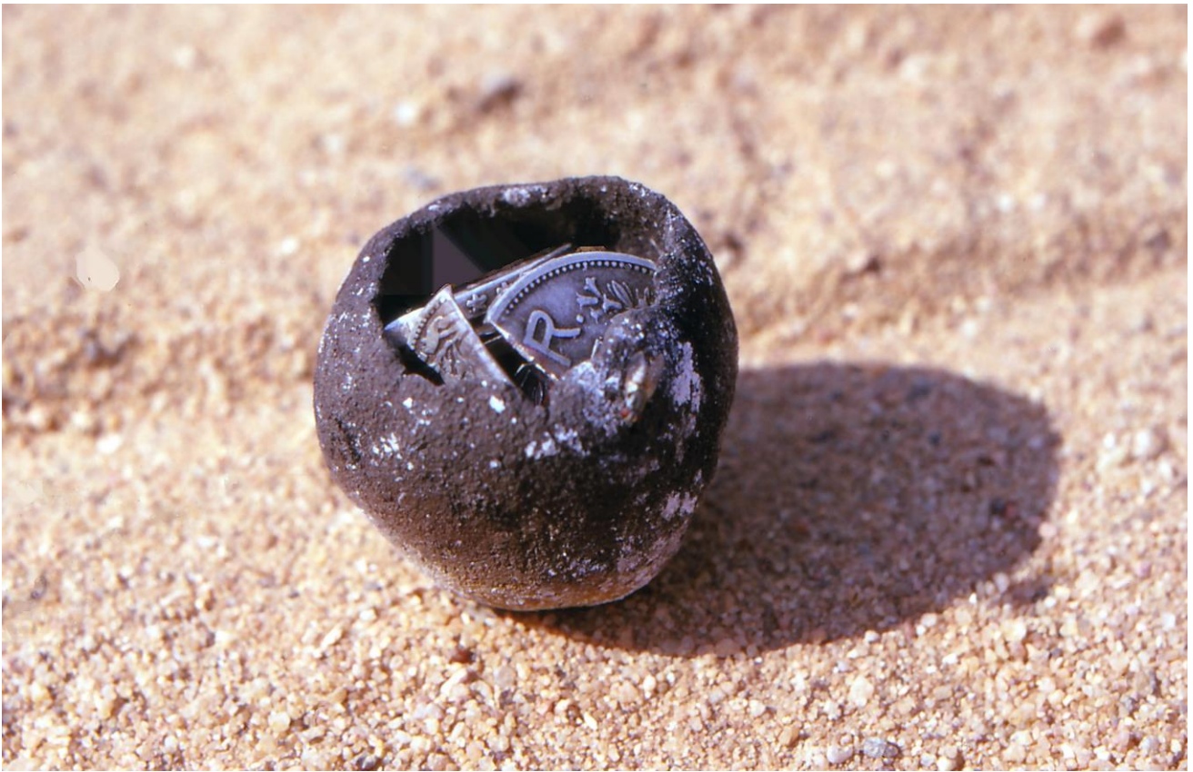
▲ Fig. 38: The small crucible is pre-fired and loaded with chopped silver coins. Next, the finished mould will be cemented onto the crucible with clay (see fig. 41).
