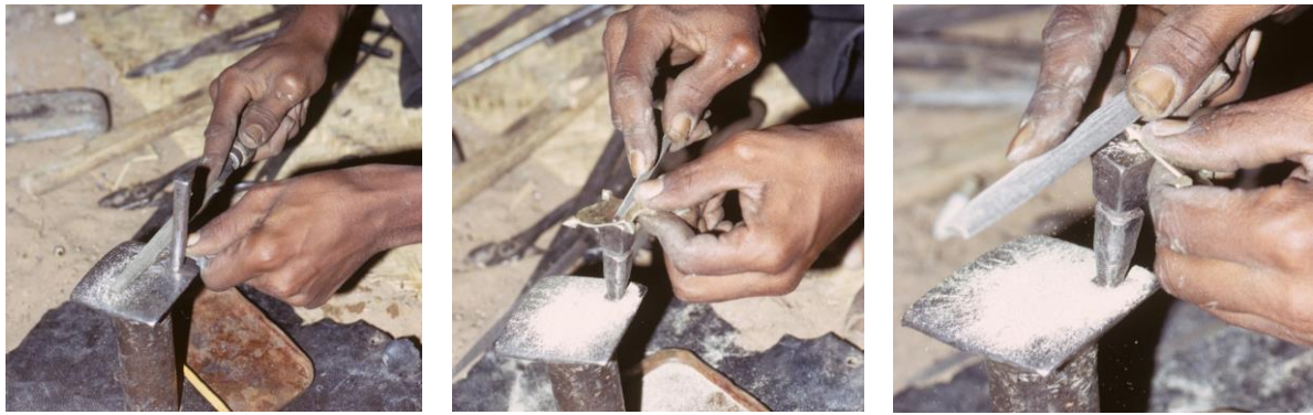
Fig. 54: Filing takes hours. The filings are valuable and are to be melted down again later. Therefore, a black collecting mat is placed around the anvil stuck in the ground. The mat is cut out of an old car hose; the anvil is part of an old car cardan shaft.
