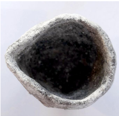
▲ Fig. 38: The small crucible is pre-fired and loaded with chopped silver coins. Next, the finished mould will be cemented onto the crucible with clay (see fig. 41).
