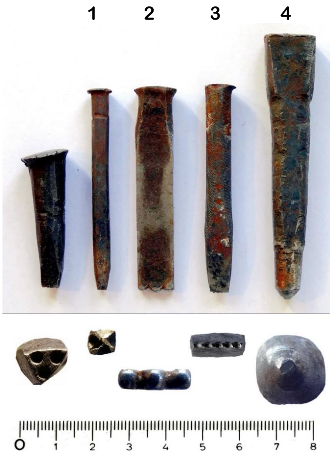
Fig. 57: Selection of decorative punches used to decorate Touareg silver jewellery. The specimen on the left comes from the Thaoua area (Niger, 1992), the others from the workshop of Hamid Kumama (Agadez, 1973):
