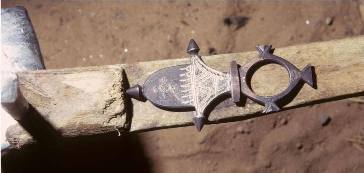
Fig. 56: Thanks to the surface being darkened in the fire, the work with the tremolo graver can be easily observed. A small board with a step (left) serves as a handle in which the jewel sits. The small board – the engraving aid – finds support in a mandrel inserted in the anvil (outside left) during vigorous engraving.
