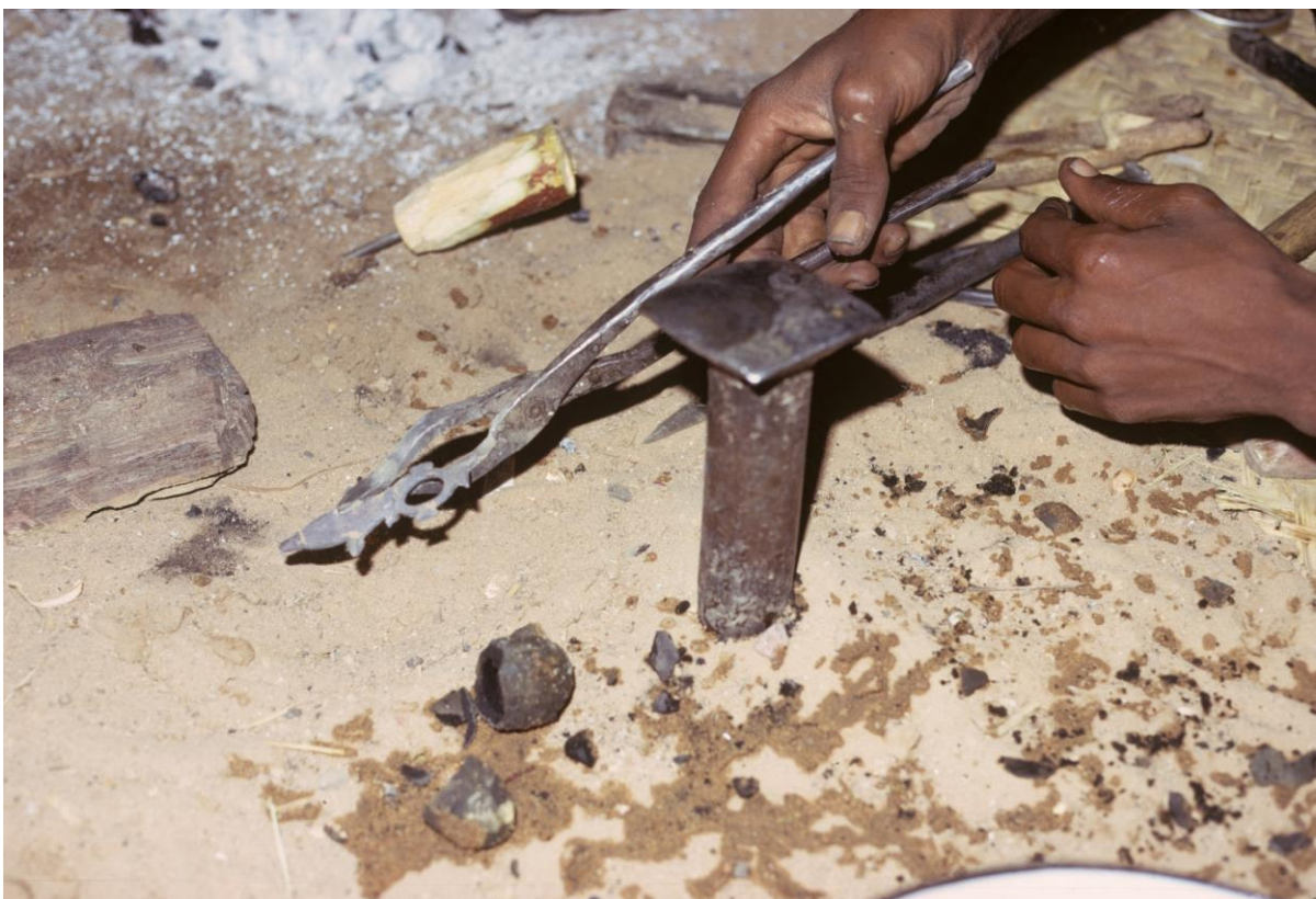
Fig. 51: In order for the red-hot piece to recrystallise homogeneously, it is not quenched in water but placed in the sand of the workshop floor and allowed to cool slowly there. The crucible and the fragments of the mould lie on the floor in front.
