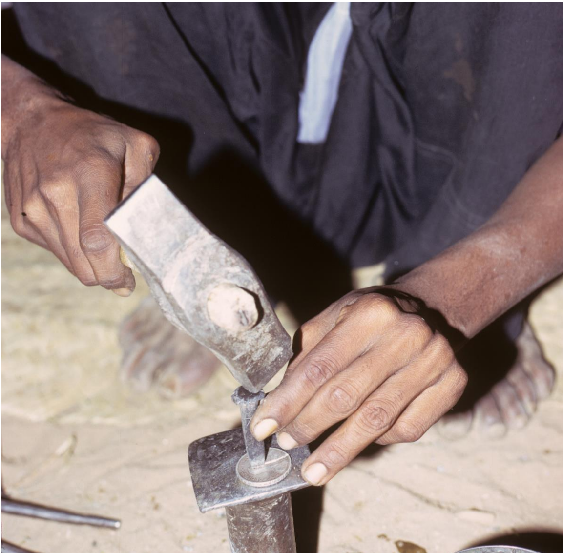
Fig. 34: Now it's time to fill the crucible with silver. We have brought along pieces of Swiss silver francs to be remelted. These have to be crushed with a chisel on the anvil so that they fit into the small crucible.
