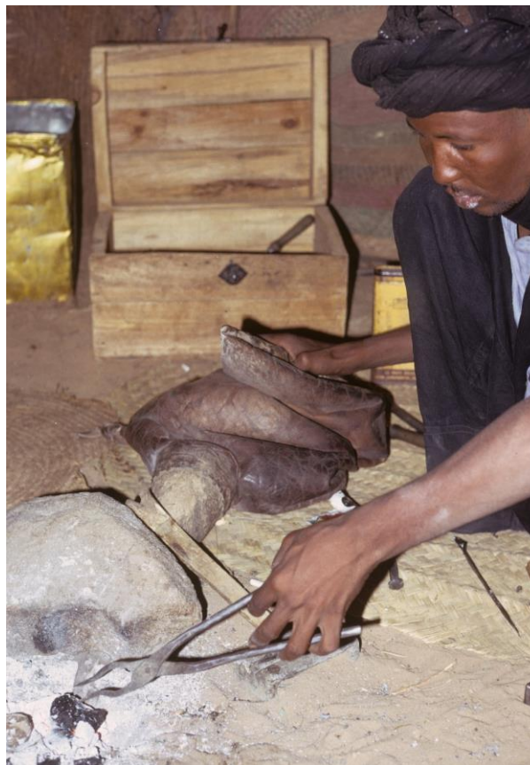
Fig. 30: The clay mould is gently heated in the fire, and the crucible (Figs. 38 and 39), which has also been formed from clay in the meantime, is dried and pre-fired.
