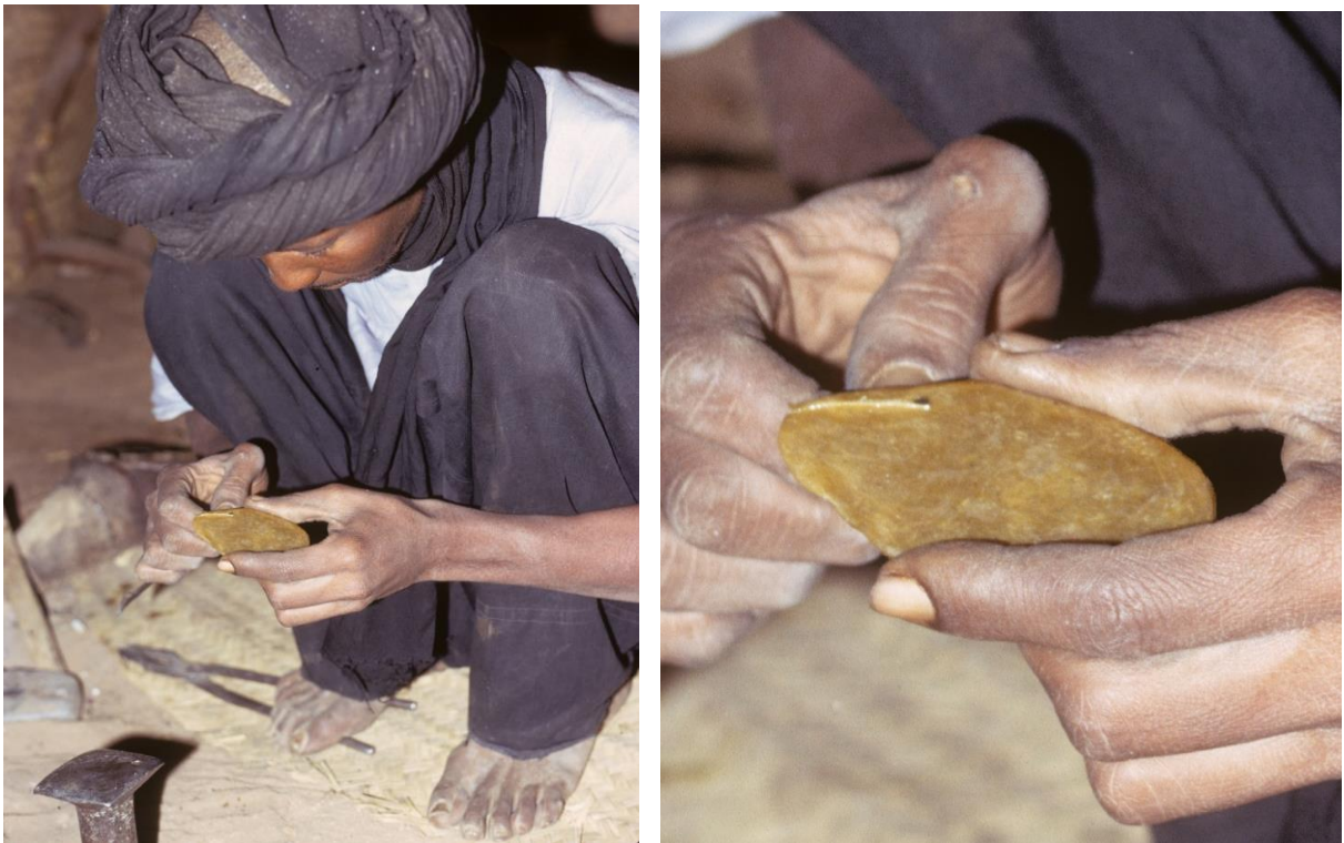
Fig. 21: Agadez, 1973: The first step is to make the positive model of an Iférouane cross from beeswax, which is later encased in a clay mould in the "lost wax process", then melted out of the mould and finally cast in silver in the cavity. The contours of the moulded wax platelet are cut out with a small metal spatula heated in the fire. (On the production process in general, see also Furger 2017A, 79 fig. 130)
