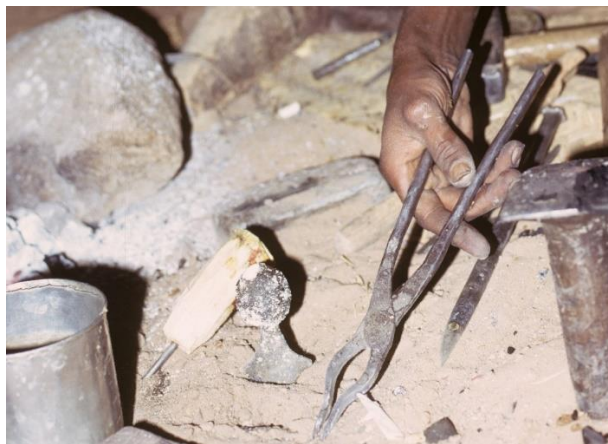
Fig. 45: First, still gentle cooling: The hot mould, with the empty crucible on top, is placed in the sand of the workshop floor (centre of picture) and cooled for a few minutes in the air.
