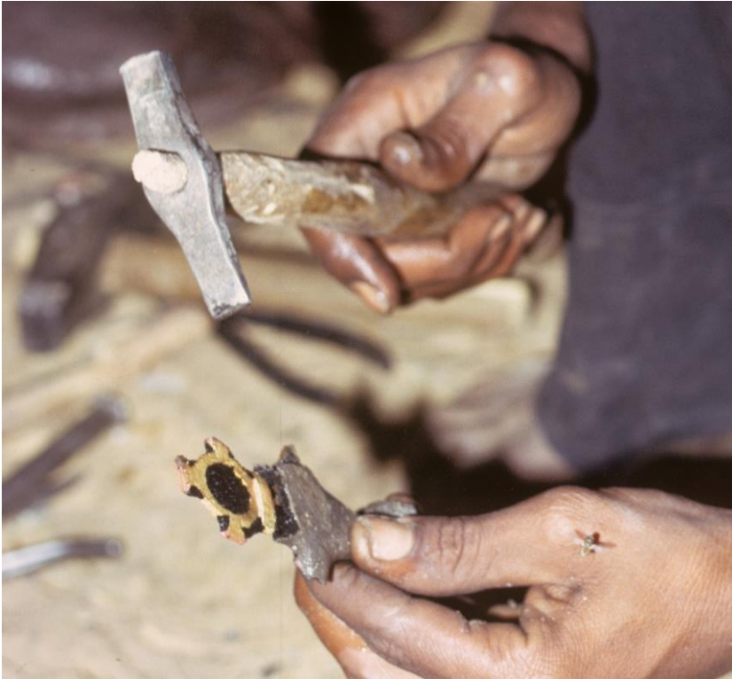
Fig. 47: The second highlight in the traditional production of a Touareg cross using the wax melting process: The clay mould is knocked away with a hammer and the casting emerges: casting successful! (Casting failures occur when, for example, the metal solidifies too early due to insufficient temperature before it has completely filled the cavity). The term "lost wax casting process" becomes obvious: the mould can only be used once; each wax model leads to a unique piece.
