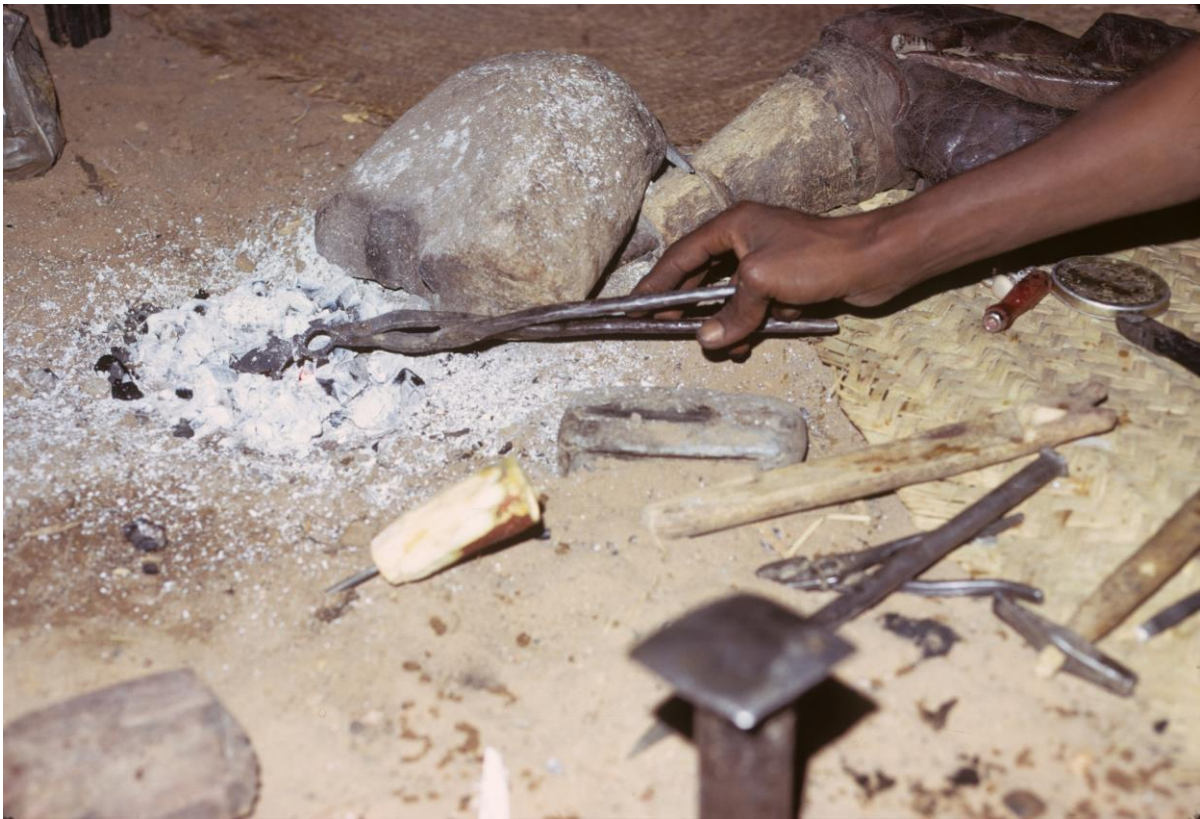
Fig. 50: The raw casting is briefly annealed in the charcoal fire (dark red) so that the casting structure of the silver alloy is homogenised. (On this recrystallisation process, see also Furger 2017B, 29 f. fig. 3).
