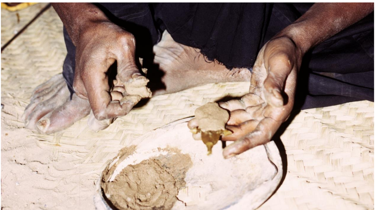
Fig. 25: The hand-modelled casting model made of beeswax is finished and covered with clay, which will later form the fireproof mould. Note the thin sprue, also moulded in wax, at the lower end of the cross. Hamid uses "his" clay directly from the ground outside his workshop.
