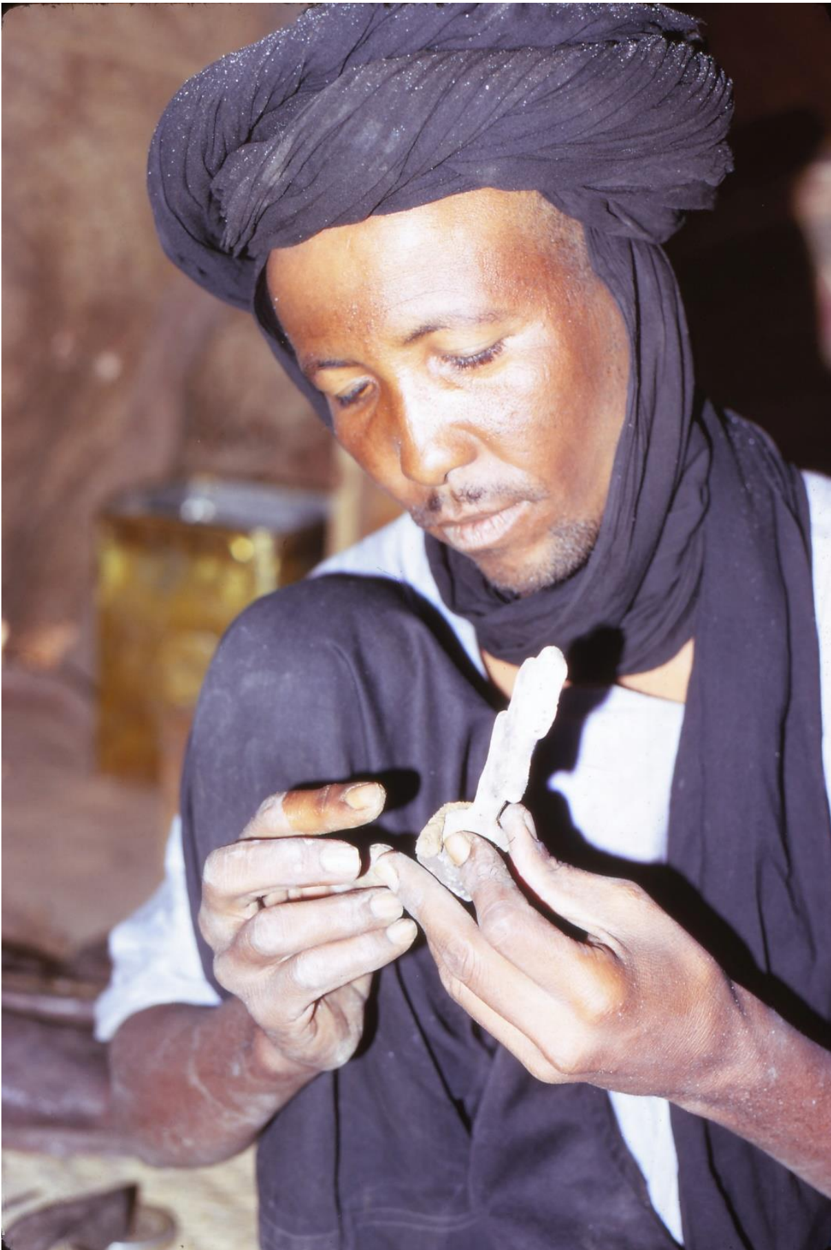
Fig. 41: Hamid Kumama connecting the crucible filled with silver chunks (below) to the mould (above) with wet clay. See figs. 37 and 40.
