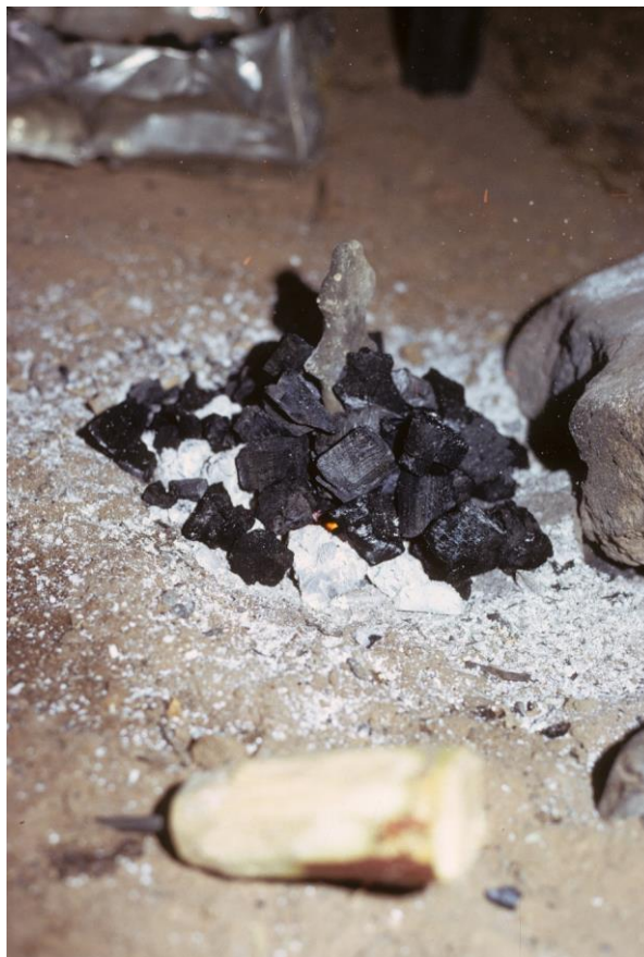
Fig. 42: Now – for the actual casting – the fire must be stoked to particularly high heat. A lot of charcoal is put on (left) and the bag bellow is started up vigorously (right).
