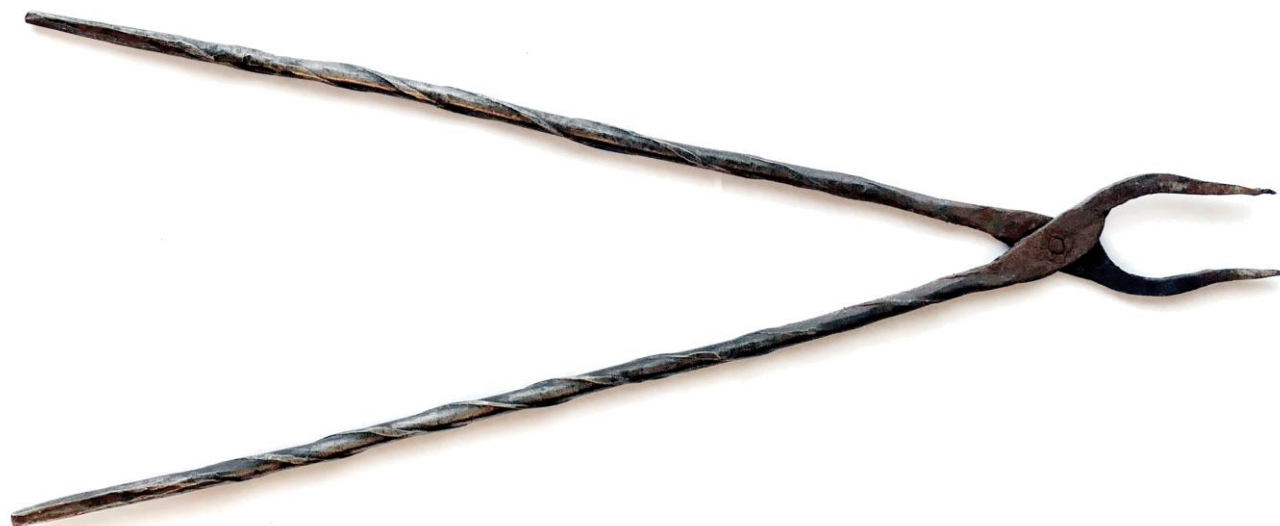
Fig. 31: Small fire tongs for fine forging of silver jewellery and for holding red-hot crucibles, moulds and lumps of charcoal. Made by Hamid Kumama from thin reinforcing iron. Length: 36 cm.
