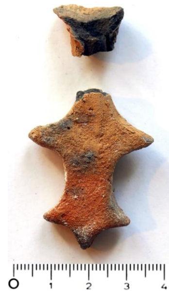
Fig. 48: Another "Cire-perdu" mould after primary firing of the clay. It is fired but empty inside. Because it broke during firing (fig. 40), it could no longer be used for casting – all the work on the wax model and mould making was in vain! Natural size.
