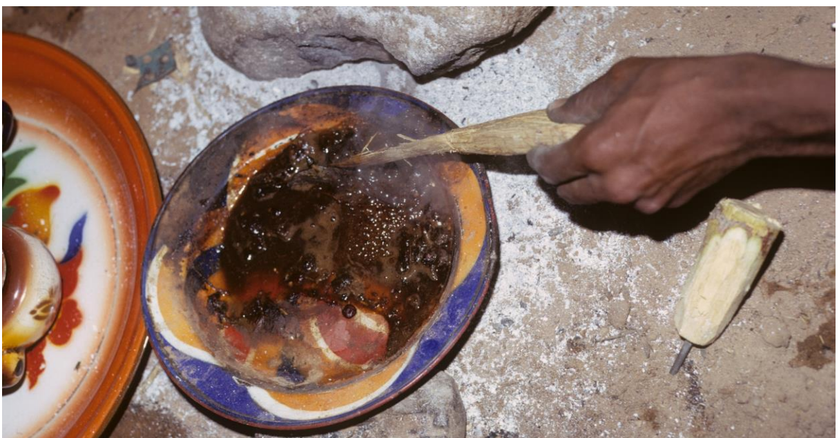
Fig. 58: After filing, grinding, engraving and hallmarking, the shape and ornamentation of the piece of jewellery are actually finished. The silver alloy of a good 80% fineness is very hard and resistant, but its colour tends slightly towards light grey. To increase the fineness and thus the shine of the silver on the surface of the object, the copper is dissolved away in an acid. This process is called "white boiling". The Touareg silversmiths used to use the boiled juice of tamarind pods as an acid. These are boiled up and crushed and squeezed with a wooden stick.
