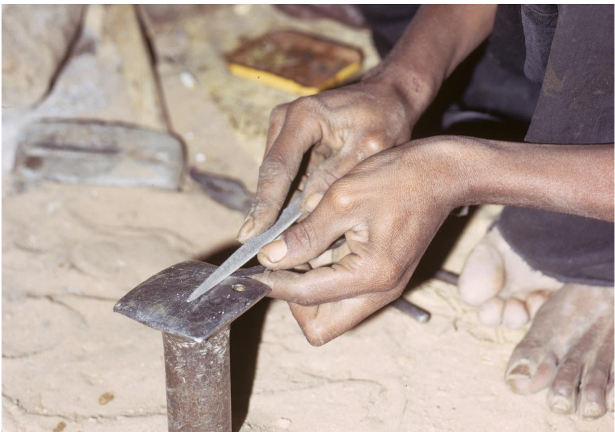
Fig. 22: The wax spatula is sharpened with the file in between.
