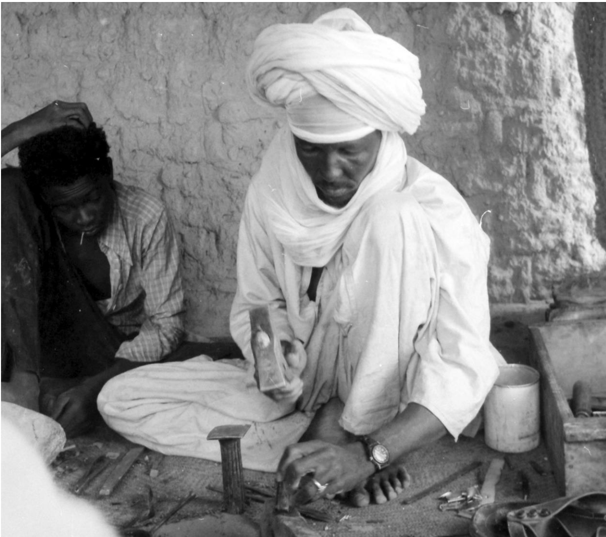
Fig. 8: Hamid Kumama 1981, in the workshop beating a little piece of sheet metal.
