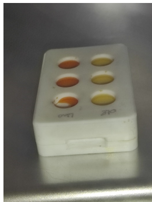
Figure 4.3: Discoloration of both \mathbf{Zr}_{12} -oleate (right) and \mathbf{Zr}_{12} -linoleate (left) to light yellow and dark orange respectively after 24h of thermal polymerisation via heating at 180 °C under vacuum.
