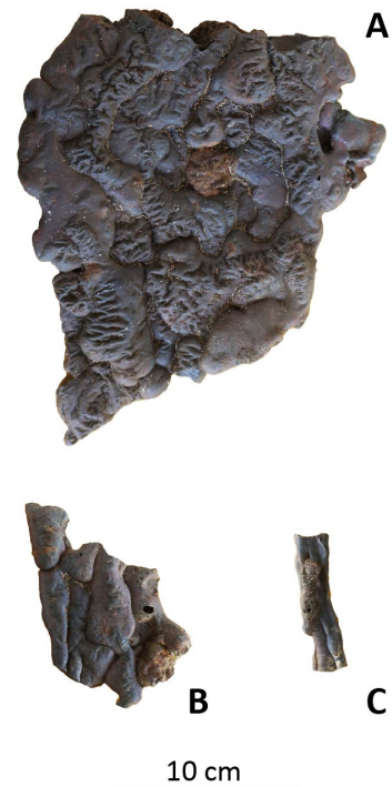
Figure 5.3: Example of three tapped slag fragments from Amboronala. A. Large slab of tapped slag overflowing out of the channel intended for the tapping of the slag. B. Typical tapped slag for northeastern Madagascar with overlapping ropy flows. C. Single flow of tapped slag.
