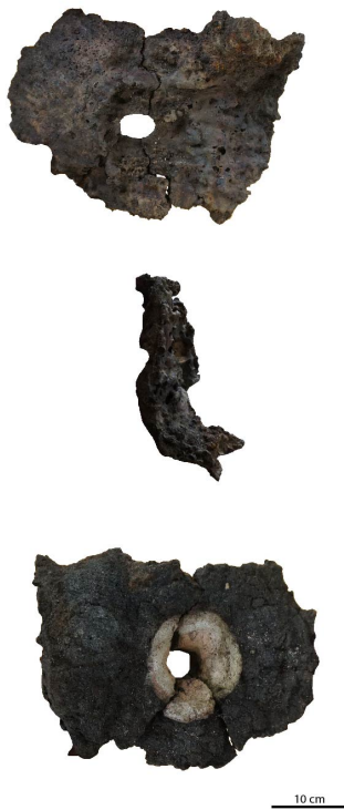
Figure 5.11: Rubbed sand wall around a clay tuyere, recovered in Amboronala. From top to bottom: Face on the hearth side; profile section of the wall; back face not in direct contact with the fire.
