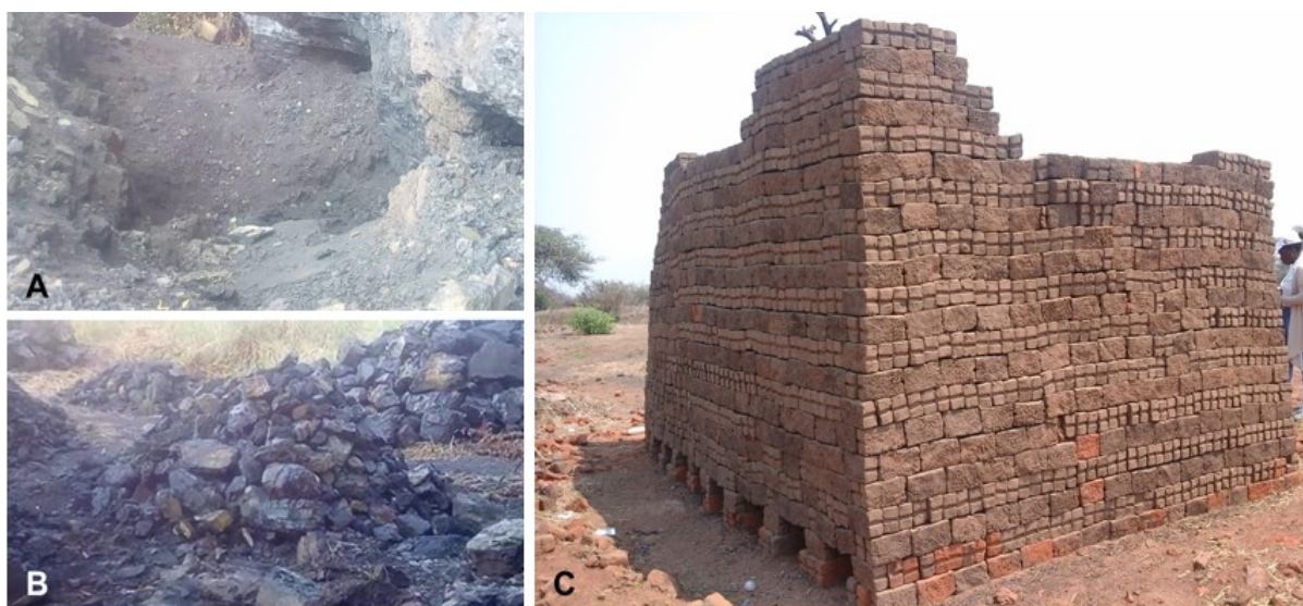
Figure 6. Artisanal coal mine for burning bricks for construction in Tete province, Mozambique. Panel A, the open pit of ASM; panel B, mined coal and panel C, artisanal bricks for housing ready to be burnt. Source: Authors
