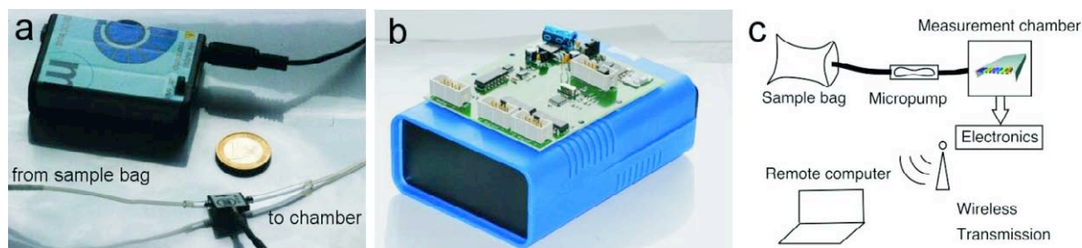
Fig. 2. (a) Battery-operated micropump system for pumping a sample of exhaled breath from a medical breath sample bag into the microcantilever measurement chamber (model mp5 from Bartels Mikrotechnik, Dortmund, Germany); (b) Bluetooth interface on top of the portable, compact and wireless measurement setup; (c) schematic of the wireless data acquisition and measurement setup.
