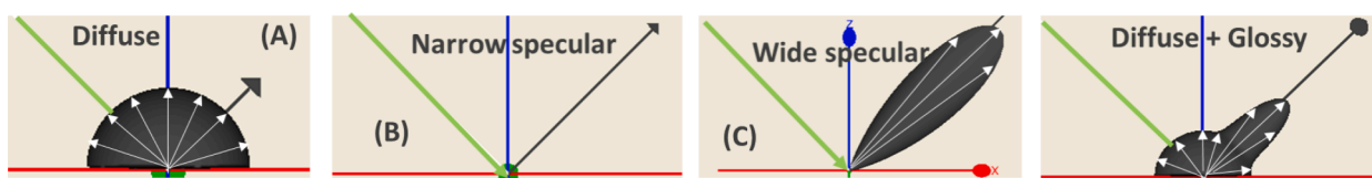
Fig. 2. The full Bidirectional Reflectivity Distribution Function (BRDF) is described as the sum of diffuse component (A) and glossy components for sharp (B) and blurry (C) components.
