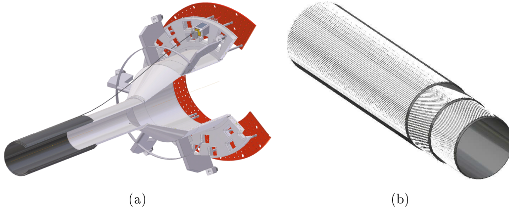
Figure 2.7: Schematic representation of the Inner Detector (ID, a) and the three scintillating fibres (b) that build up the active area of the detector. Figures taken from [262]
