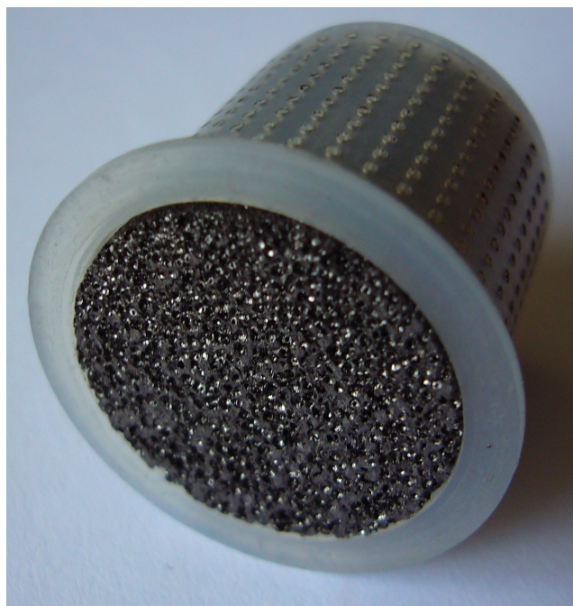
Figure 2.13: Carbon foam target. Figure taken from [287].
