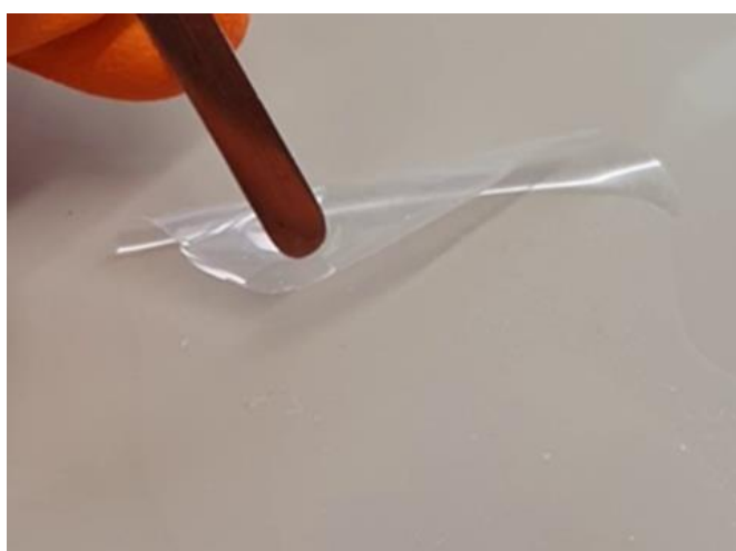
Figure S6. Picture of the self-standing thin film obtained from the self-assembled micelle solution (difficult to handle)
