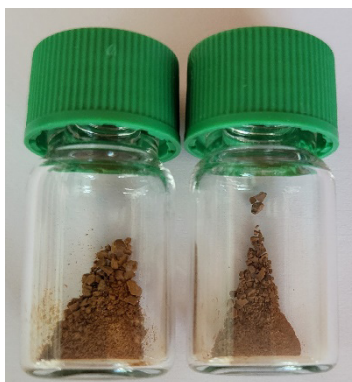
Figure 48: Dried Ru( 21 )(bpy)@TiO 2 (left) and Ru( 21 ) 2 @TiO 2 NPs (right).
