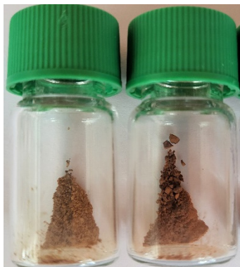
Figure 49: Dried Ru(21)(bpy)@TiO_2 (left) and Ru(21)_2@TiO_2 NPs (right) after polymerization attempt with FeCl_3 .
