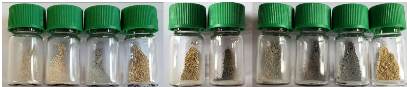
Figure 22: Isolated f-NPs; from left to right rR@SrTiO 3 , rR@SrTiO 3 -a , rR@SrTiO 3 -OH , rR@SrTiO 3 -OH-A , Ru@SrTiO 3 , Ru@BaTiO 3 , rR@BaTiO 3 -a , rR@BaTiO 3 -OH , rR@BaTiO 3 -OH-A .
