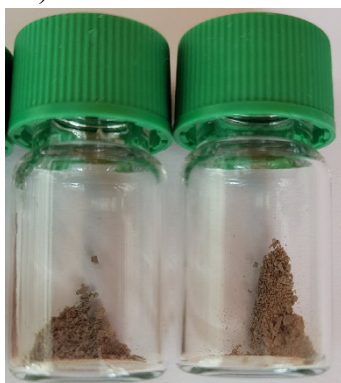
Figure 50: Dried Ru(21)(bpy)@TiO_2 (left) and Ru(21)_2@TiO_2 NPs (right) after polymerization attempt with FeCl_3 and H_2O_2 .
