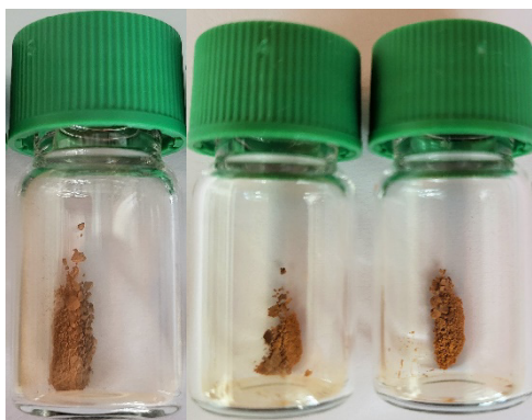
Figure 53: \text{Ru}(\mathbf{21})(\text{bpy})@\text{TiO}_2 after VPP using \text{FeCl}_3 without TTh (left) and \text{Ru}@\text{TiO}_2 after VPP with TTh using \text{FeCl}_3 (middle) or PTSa (right).
