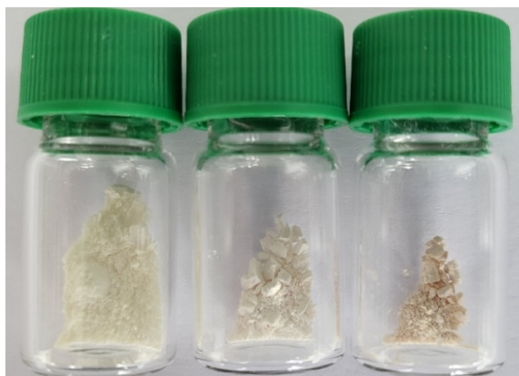
Figure 34: Photograph of commercial heat treated ZnO NPs (left), 9 @ZnO (middle) and cis -Ru(bpy) 2 Cl 2 complexed 9 @ZnO (right).
