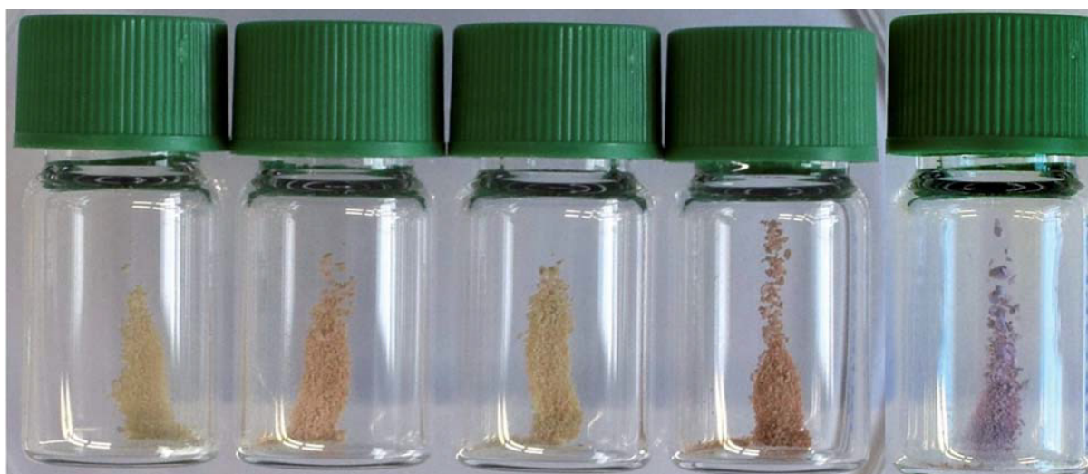
Figure 13: Photographs of activated TiO 2 NPs from left to right: functionalized with 1 and 3 ; and after treatment with [Cu( 5 ) 2 ][PF 6 ]; [Cu( 7 ) 2 ][PF 6 ]; [Cu( 6 ) 2 ][PF 6 ]; [Fe( 8 ) 2 ][PF 6 ] 2 . 17
