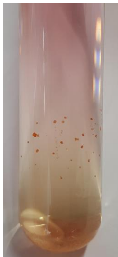
Figure 3. Crystals of a coordination polymer grown using the layering technique of solutions of a metal salt and a ligand. On top: pink methanol solution of \text{Co}(\text{NCS})_2 ; at the bottom: chloroform solution of the chosen organic ligand; single crystals formed at the interface after the two solutions started diffusing one into the other.
