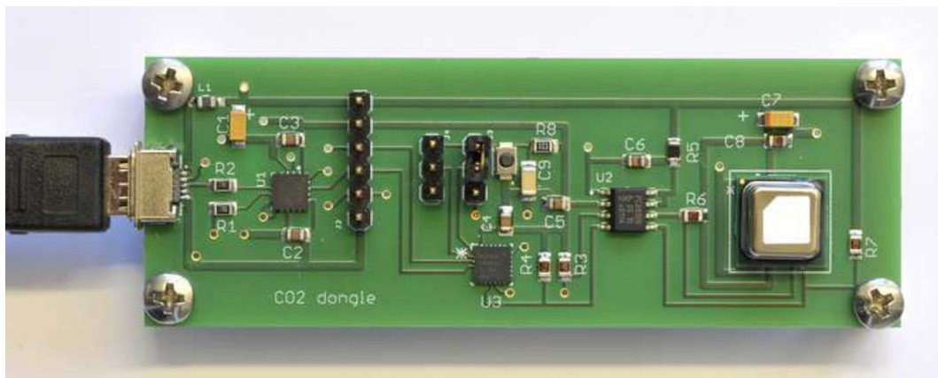
Fig. 4. Photograph of the finished dongle showing from left to right: the USB connector, USB-UART-bridge IC, microcontroller, I2C level shifter IC and the sensor with the CO 2 -permeable membrane on top.
