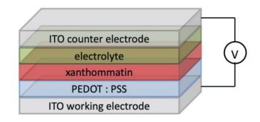
Fig. 3. Device architecture for the xanthommatin-based ECDs reported by  $\mathsf{Deravi}^{[6]}$
