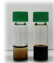
Figure 1. Photograph of \text{Cu}_3\text{N} nanocrystals after regular (left) and optimized (right) purification.
