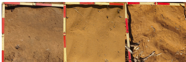
Fig. 4. Examples of the surface types: left crust (S), middle sandy deposit (G), and right loosened soil (MC).
