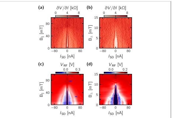
**Figure 4.** DC differential resistance (a) and (b) and RF signal (c) and (d) as a function of external magnetic field at  $V_G = -25$  V. The magnetic field is applied parallel  $(B_{\parallel})$  as well as perpendicular to the chip surface  $(B_{\perp})$ .
