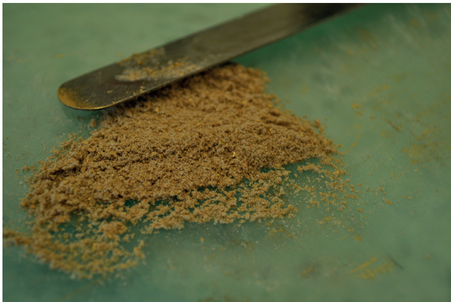
Figure 6.12: Photograph from the reconstruction of the recipe of the Liber illuministarum , showing the grey granular mass after grinding. Image © Michèle Seehafer.
