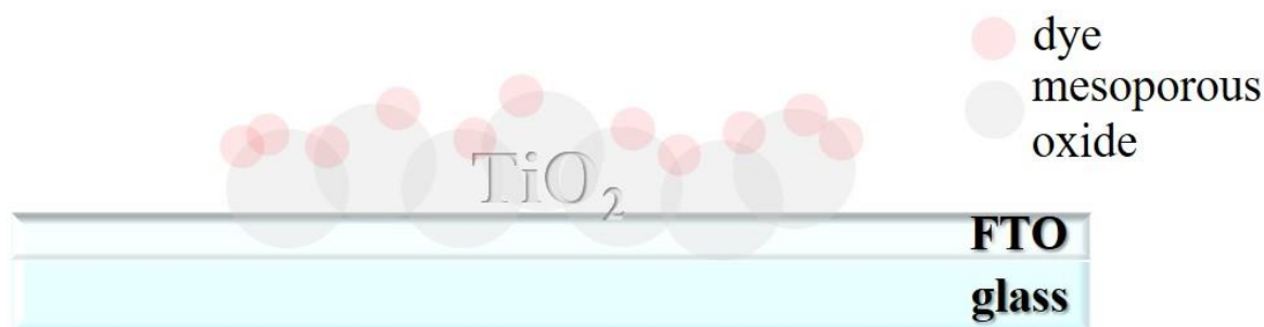
Figure 1.5. The schematic representation of working electrode.
