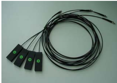
System set-up for online DO measurement in shaking flasks
