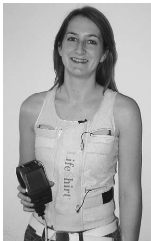
Fig. 1. The LifeShirt system: design of garment and interface with digital recorder.
