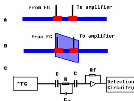
Figure 3. Schematic of the cell design for contactless conductivity detection: A) without shielding; B) with shielding; C) equivalent circuitry. FG = functional generator, C = cell capacitance, R = cell resistance,  $C_0$  = stray capacity,  $R_f$  = feedback resistor on the operational amplifier.
