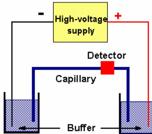
Figure 1. Structure of capillary electrophoresis
