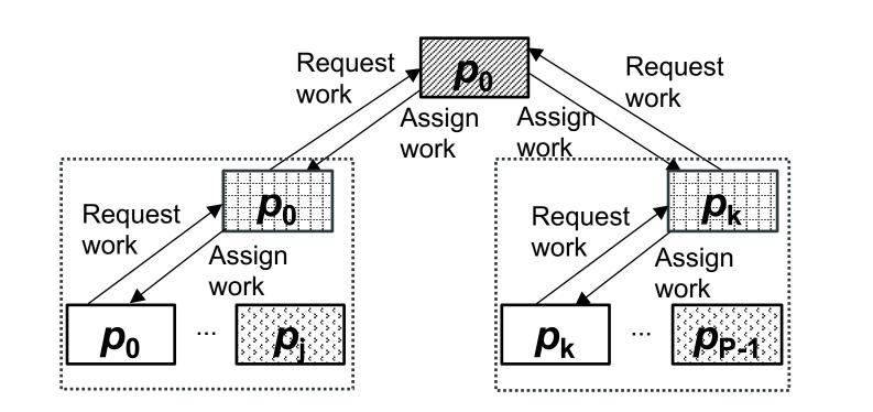
Hierarchical master-worker model using hybrid MPI two-sided communications and OpenMP. Local masters are distributed across multiple physical compute nodes [4].
