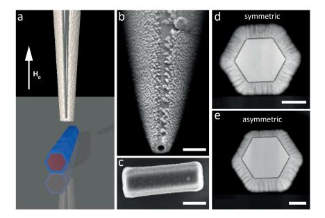
Figure 1. Experimental setup. (a) Schematic drawing showing the scanning SOT, a FNT lying on the substrate, and the direction of  $H_0$ . The CoFeB shell is depicted in blue and the GaAs core in red. Pb on the SOT is shown in white. SEMs of the (b) the SOT tip and (c) a 0.7- $\mu$ m-long FNT. (d) and (e) show cross-sectional HAADF STEMs of two FNTs from a similar growth batch as those measured. The scalebars represent 200 nm in (b) and (c) and 50 nm in (d) and (e).
