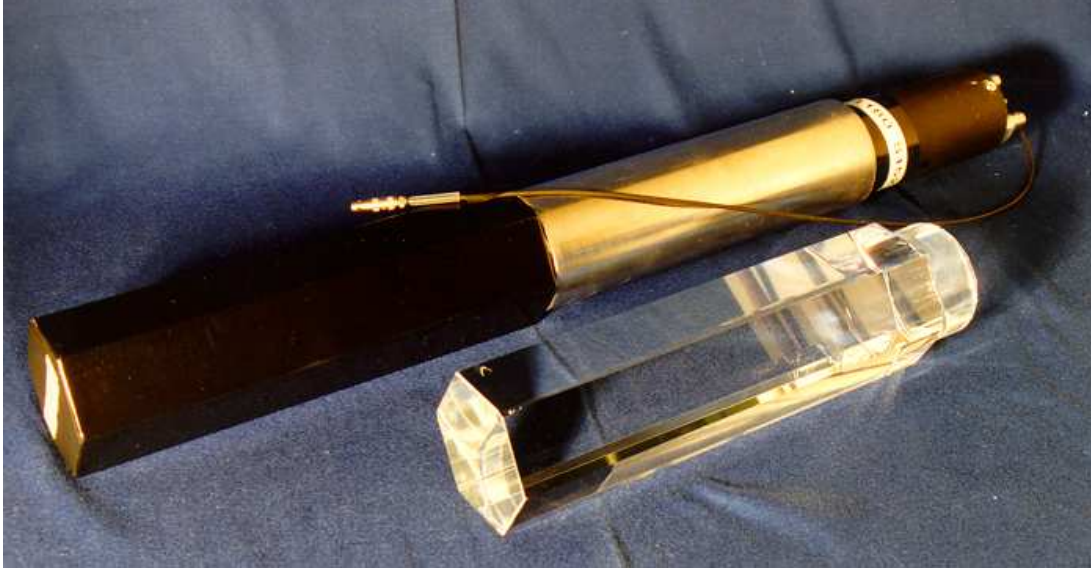
Figure 2.6: picture of a single BaF 2 crystal and a fully mounted detector element with its photomultiplier where the crystal is covered with black tape
