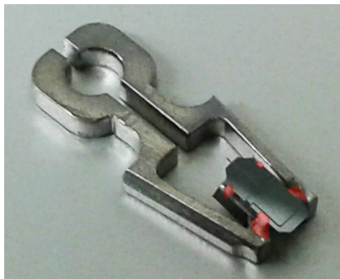
Figure 3.11.: Holder with cantilever, which was glued with the four point technique to ensure high Q -factor on the first and second resonance. The spots of the epoxy glue are marked in red.
