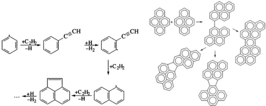
**Fig. 1.** *Left:* growth of PAHs according to the H abstraction- $C_2H_2$  addition (HACA) mechanism proposed by Frenklach *et al.* (1984). *Right:* growth of aromatic structures via the dimerisation and coalescence of PAHs proposed by Mukherjee *et al.* (1994).
