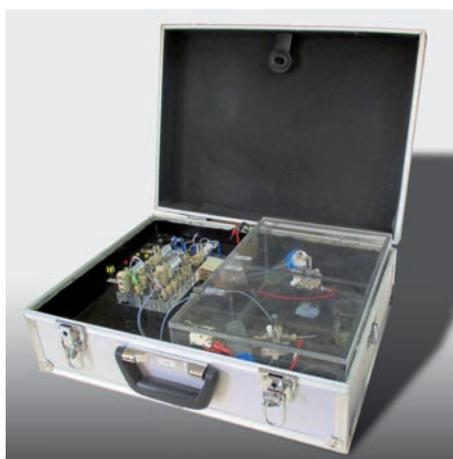
Fig. 3. Photograph of the dual-channel portable CE system.<sup>[7]</sup>
