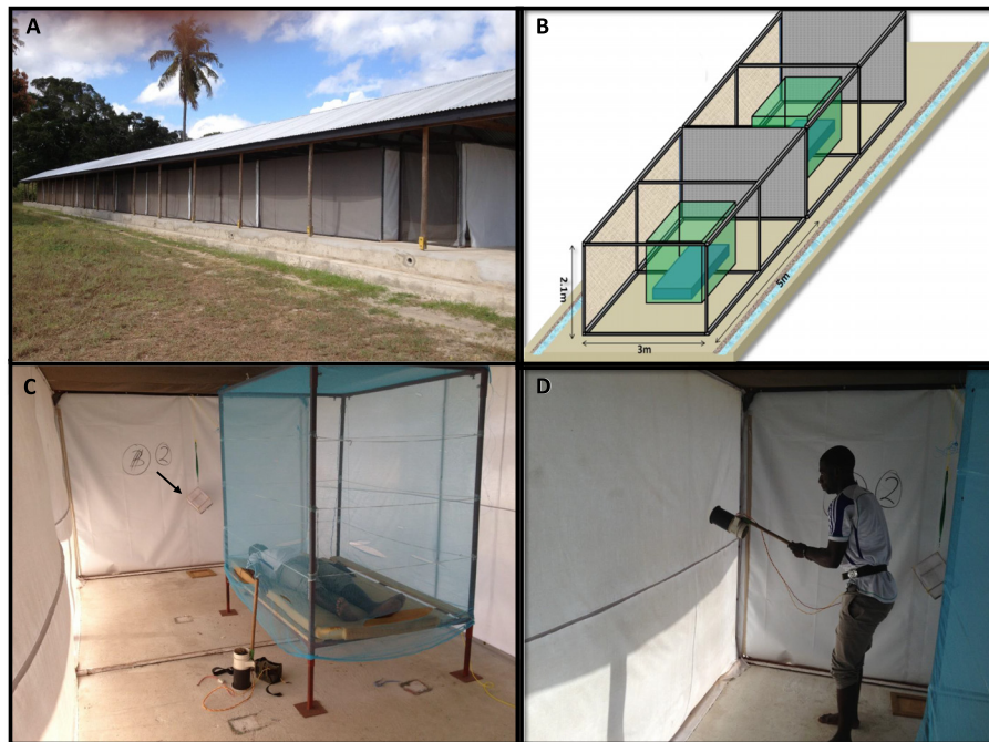
Figure 4 Experimental set-up in the Ifakara Tunnel Test (ITT). Ifakara Tunnel situated at Bagamoyo Research Training Centre (BRTC) in Kingani, Bagamoyo. The tunnel is a 50 m long, 3 m wide and 2.1 m high steel tube frame construction upon a concrete base surrounded by a water channel and beneath a beamed wooden frame supporting a corrugated steel roof (A). Net covered tunnel divided into 10 individual compartments containing bed and adjustable steel net frame (B). Experimental set up for Ifakara Tunnel Test. A human volunteer will sleep beneath the LLIN from 21.00 hrs to 06.00 hrs. Anopheles gambiae mosquitoes will be released from the holding cages by raising a cage from its wooden base (arrow) using a nylon string (C). At the end of the experiment, all mosquitoes within each of the compartments will be removed with a Prokopack (D).
