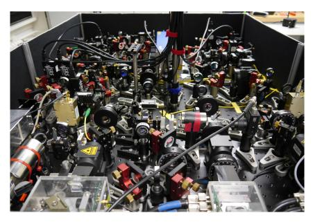
Figure A.7: View over the laser system. The lasers on the bottom are stabilized using saturated absorption spectroscopy, amplified and distributed into fibers.
