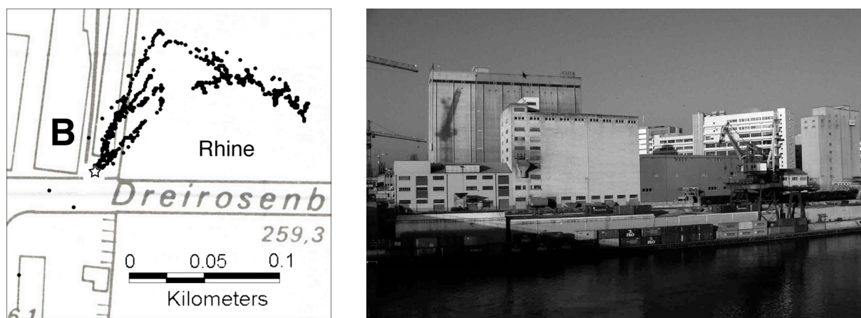
Figure 1: On the left, we show an example of a GPS test performed on 22 April 2003 at the bridge Dreirosenbrücke. The star on the map indicates the real position of the stationary GPS receiver during the test. The reflection on the high buildings of the Rhine harbour St Johann (B) caused shifted positions (the points over the river). On the right, we show a view of the high buildings of the harbour.
