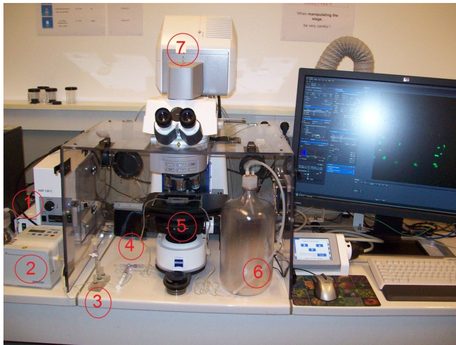
Figure 50: Picture of the complete experimental setup: (1) bottle with the bacteria nutritive medium, (2) peristaltic pump, (3) bubble trap, (4) injection system (syringe and adequate connector), (5) home-made flow cell, (6) trash bottle (bacteria nutritive medium after culture) and (7) Zeiss LSM700 confocal microscope.
