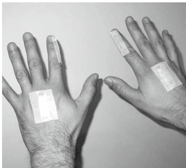
Figure 2. Position of the TLDs on the index fingers and backs of hands.
