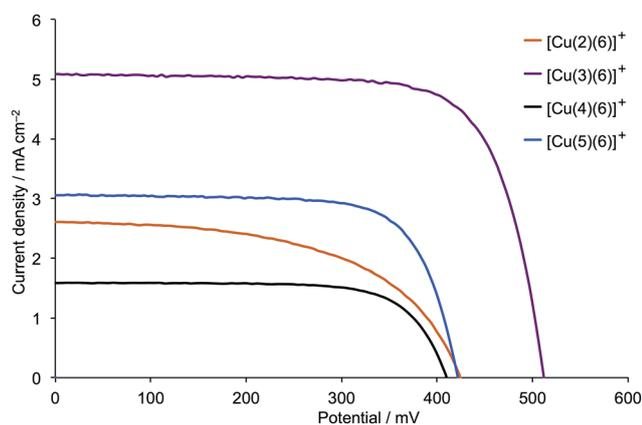
**Fig. 3**  $J$ - $V$  curves for DSCs containing [Cu(2)(6)]<sup>+</sup>, [Cu(3)(6)]<sup>+</sup>, [Cu(4)(6)]<sup>+</sup> and [Cu(5)(6)]<sup>+</sup> combined with  $I_3^-/I^-$  electrolyte. For data for duplicate DSCs, see Fig. S5.†
