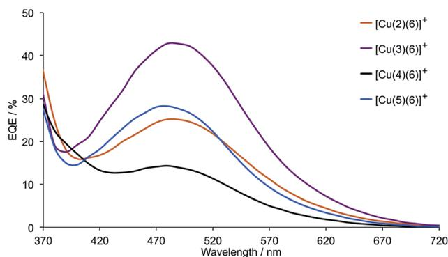
**Fig. 4** EQE spectra for DSCs containing dyes [Cu(2)(6)]<sup>+</sup>, [Cu(3)(6)]<sup>+</sup>, [Cu(4)(6)]<sup>+</sup> and [Cu(5)(6)]<sup>+</sup> combined with  $I_3^-/I^-$  electrolyte. For spectra for duplicate DSCs, see Fig. S7.†
