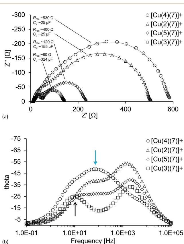
Fig. 7 (a) Nyquist plots and (b) Bode plots for DSCs containing the dyes  $[\text{Cu}(2)(7)]^+$ ,  $[\text{Cu}(3)(7)]^+$ ,  $[\text{Cu}(4)(7)]^+$  and  $[\text{Cu}(5)(7)]^+$ . See text for interpretation of the blue and black arrows.
