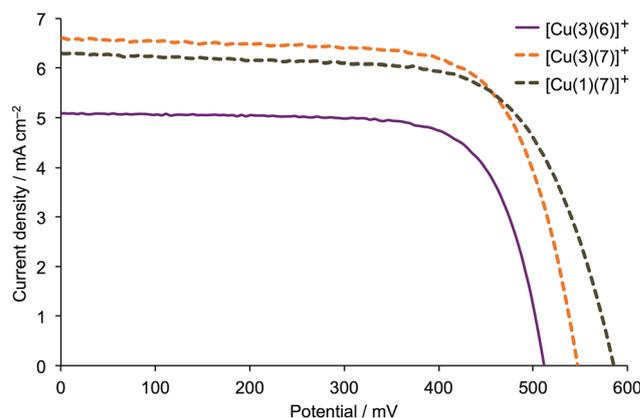
Fig. 5  $J$ - $V$  curves for DSCs containing  $[\text{Cu}(3)(6)]^+$ ,  $[\text{Cu}(3)(7)]^+$  and  $[\text{Cu}(1)(7)]^+$  combined with  $\text{I}_3^-/\text{I}^-$  electrolyte. For data for duplicate DSCs with  $[\text{Cu}(3)(7)]^+$  and  $[\text{Cu}(1)(7)]^+$ , see Fig. S10†
